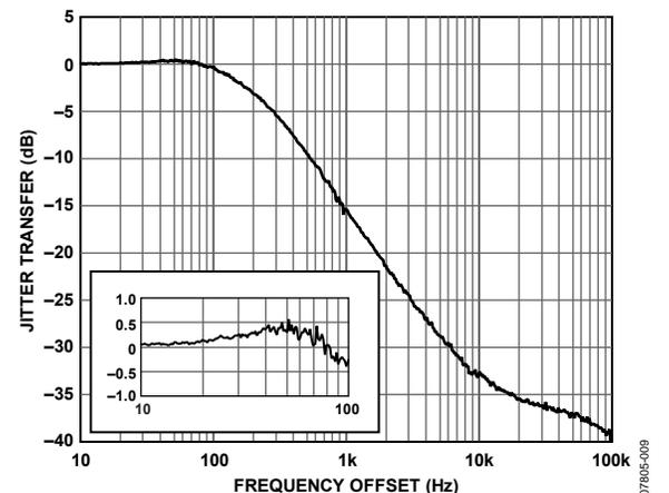
Figure 9. Jitter Transfer (Nominal Peaking)
