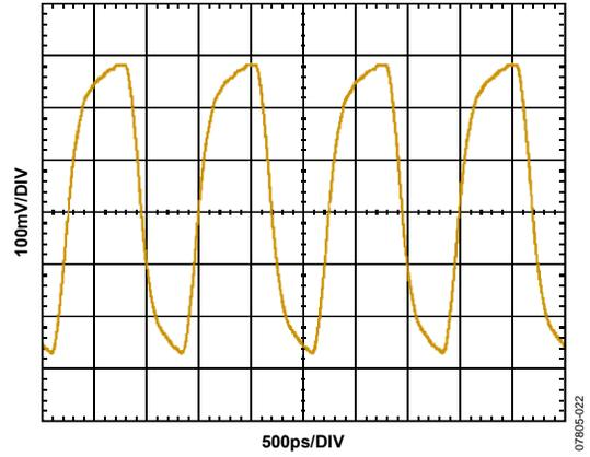
Figure 18. Typical Output Waveform—LVDS (805 MHz, 3.5 mA Drive Current)
