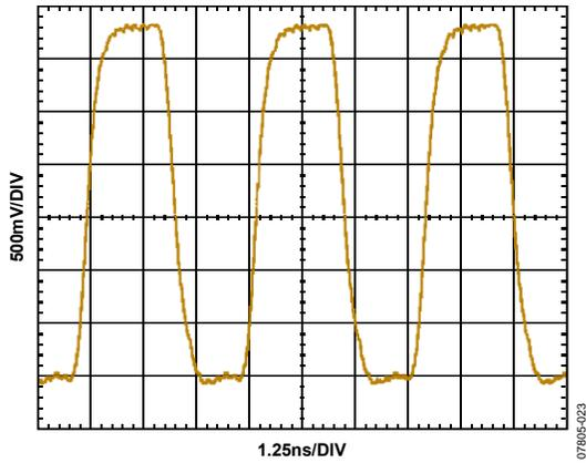
Figure 17. Typical Output Waveform—CMOS (250 MHz, 10 pF Load)
