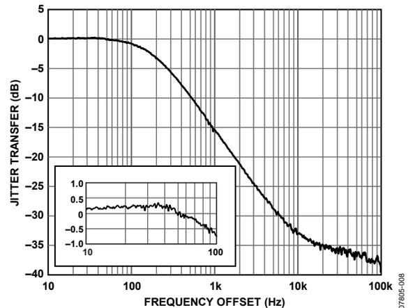
Figure 6. Jitter Transfer (Minimal Peaking)
