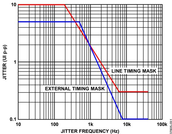
Figure 22. Jitter Tolerance
