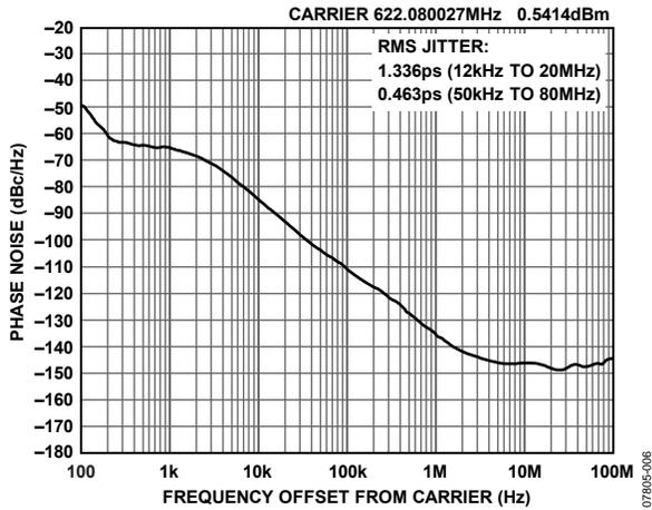
Figure 5. Phase Noise, 19.44 MHz Mode, Fractional-N
