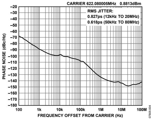
Figure 4. Phase Noise, Fractional-N
