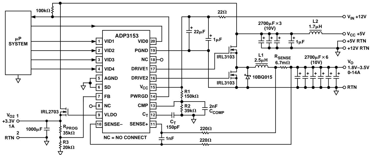
Figure 2. Typical VRM8.2 Compliant Core DC/DC Converter Circuit
