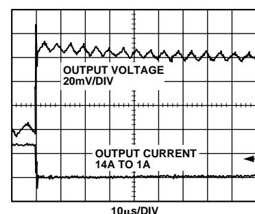
Figure 9. Transient Response, 14 A-1A of Figure 2 Circuit
