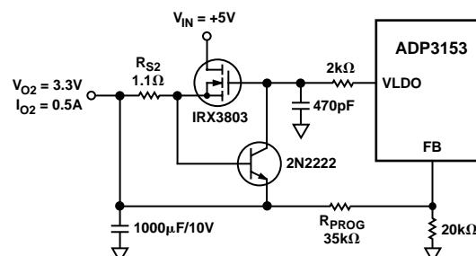
Figure 14. Linear Regulator with Overcurrent Protection
