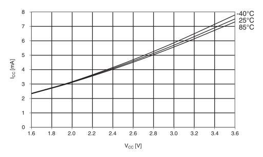
Figure 33-49. Active supply current vs.  $V_{CC}$ .  $f_{SYS} = 32MHz internal RC$ .
