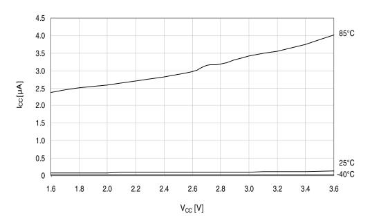
Figure 33-234. Power-down mode supply current vs. V<sub>CC</sub>. Watchdog and sampled BOD enabled.
