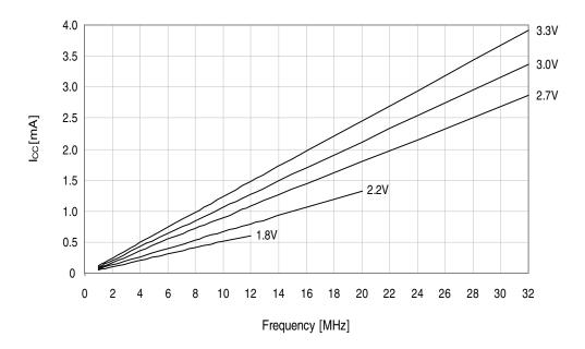
Figure 33-161. Idle mode supply current vs.  $V_{CC}$ .  $f_{SYS} = 32.768kHz$  internal oscillator.
