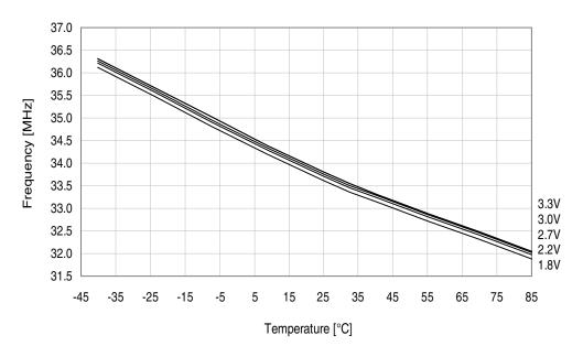
Figure 33-345. 32MHz internal oscillator frequency vs. temperature.
