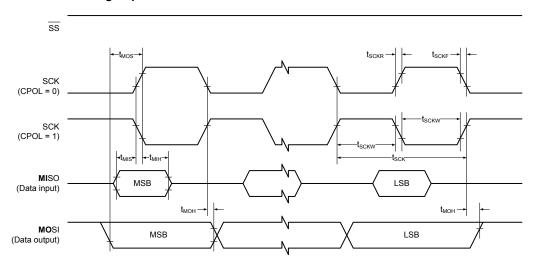
Figure 32-6. SPI timing requirements in slave mode.
