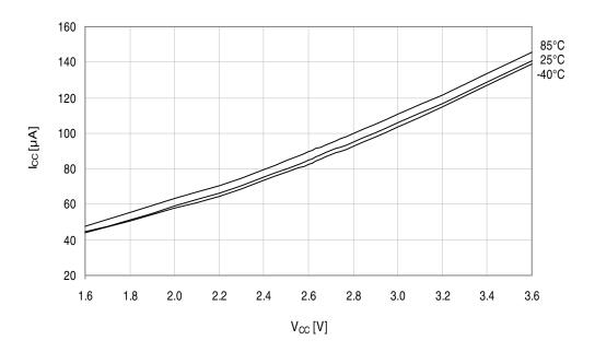
Figure 33-230. Idle mode supply current vs.  $V_{CC}$ .  $f_{SYS} = 2MHz$  internal oscillator.
