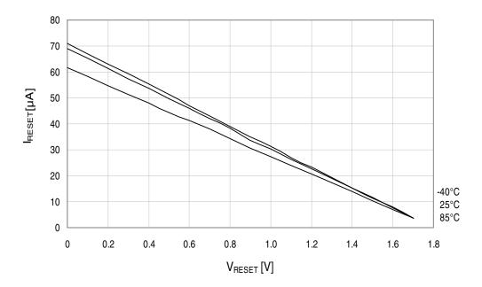
Figure 33-268. Reset pin pull-up resistor current vs. reset pin voltage.  $V_{CC} = 3.0V$ .
