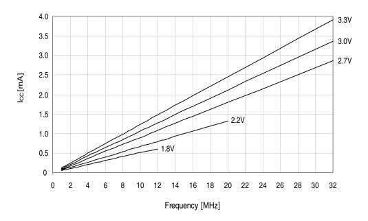
Figure 33-228. Idle mode supply current vs.  $V_{CC}$ .  $f_{SYS} = 32.768kHz$  internal oscillator.
