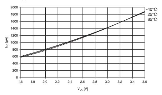
Figure 33-48. Active supply current vs.  $V_{CC}$ .  $f_{SYS} = 32MHz internal RC prescaled to 8MHz.$
