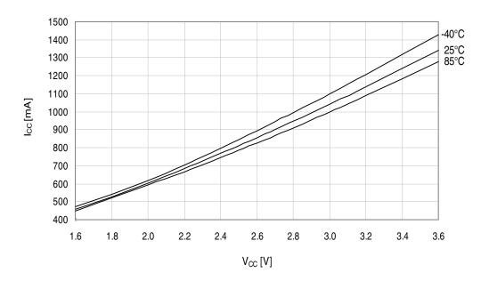
Figure 33-157. Active mode supply current vs.  $V_{CC}$ .  $f_{SYS} = 32MHz$  internal oscillator prescaled to 8MHz.
