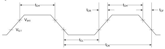
Table 32-168.External clock used as system clock without prescaling.
