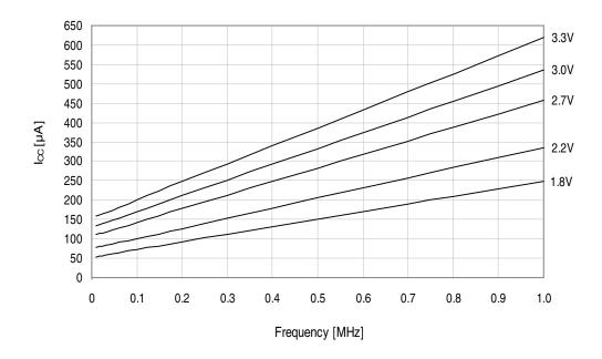
Figure 33-220. Active supply current vs. frequency.  $f_{SYS} = 1 - 32MHz$  external clock,  $T = 25^{\circ}C$ .
