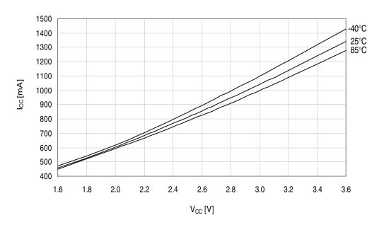
Figure 33-224. Active mode supply current vs.  $V_{CC}$ .  $f_{SYS} = 32MHz \ internal \ oscillator \ prescaled \ to \ 8MHz.$
