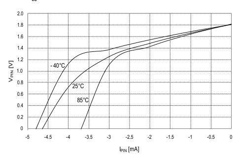
Figure 33-106. I/O pin output voltage vs. source current.  $V_{CC} = 3.0V$ .
