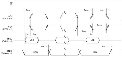
Figure 32-13.SPI timing requirements in slave mode.
