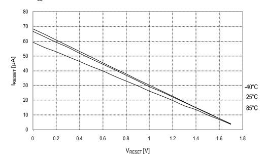
Figure 33-134. Reset pin pull-up resistor current vs. reset pin voltage.  $V_{CC}$  = 3.0V.
