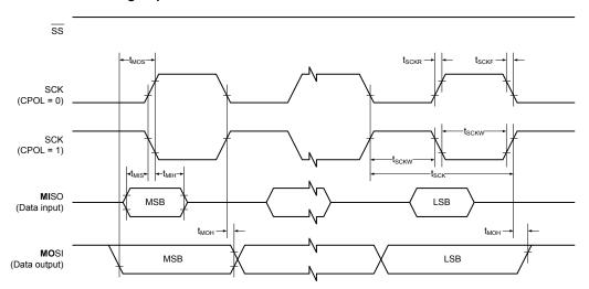
Figure 32-27. SPI timing requirements in slave mode.
