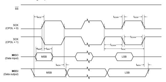
Figure 32-34. SPI timing requirements in slave mode.
