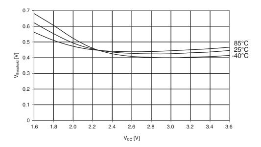
Figure 33-30. Reset input threshold voltage vs.  $V_{CC}$ .  $V_{/L}$  - I/O pin read as "1".
