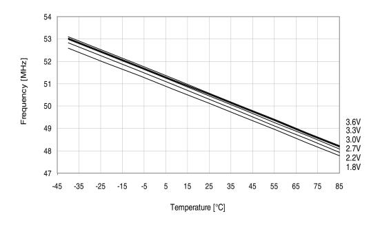
Figure 33-282. 48MHz internal oscillator frequency vs. temperature.
