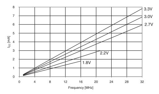
Figure 33-52. Idle supply current vs.  $V_{CC}$ .  $f_{SYS} = 1.0MHz$  external clock.
