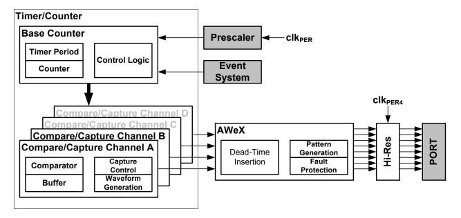
PORTC has one Timer/Counter 0 and one Timer/Counter1. PORTD, PORTE and PORTF each has one Timer/Counter 0. Notation of these are TCC0 (Time/Counter C0), TCC1, TCD0, TCE0, and TCF0, respectively.
