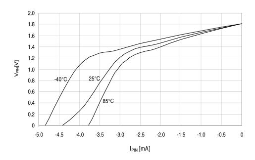
Figure 33-173. I/O pin output voltage vs. source current.  $V_{CC} = 3.0V$ .
