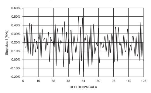
Figure 33-38. Internal 32MHz oscillator CALB calibration step size. T = -40 to  $85^{\circ}$ C,  $V_{CC} = 3V$ .
