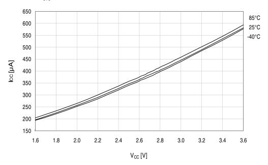
Figure 33-291. Active mode supply current vs.  $V_{CC}$ .  $f_{SYS} = 32MHz internal oscillator prescaled to 8MHz.$
