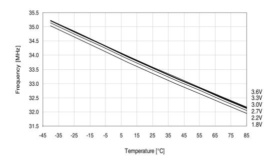
Figure 33-278. 32MHz internal oscillator frequency vs. temperature.
