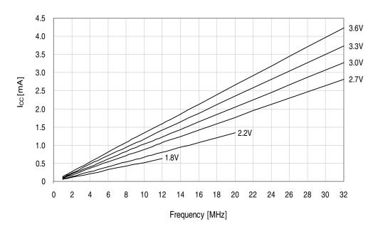
Figure 33-295. Idle mode supply current vs.  $V_{CC}$ .  $f_{SYS} = 32.768kHz$  internal oscillator.
