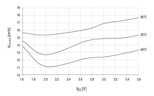
Figure 33-193. Analog comparator hysteresis vs. V<sub>CC</sub>. *Large hysteresis*.
