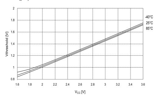
Figure 33-112. I/O pin input threshold voltage vs.  $V_{CC}$ .  $V_{IL}$  I/O pin read as "0".
