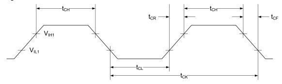
Table 32-139.External clock used as system clock without prescaling.
