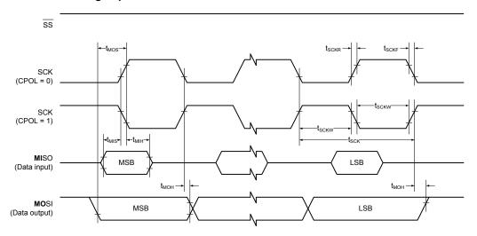
Figure 32-20.SPI timing requirements in slave mode.
