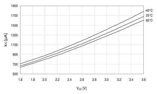
Figure 33-299. Idle mode current vs.  $V_{CC}$ .  $f_{SYS} = 32MHz$  internal oscillator.
