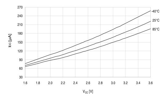
Figure 33-155. Active mode supply current vs.  $V_{CC}$ .  $f_{SYS} = 1MHz \ external \ clock$ .
