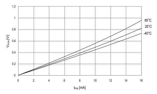
Figure 33-110. I/O pin output voltage vs. sink current.
