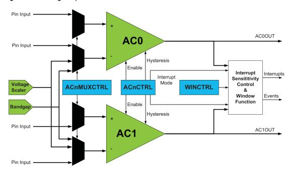
The window function is realized by connecting the external inputs of the two analog comparators in a pair as shown in Figure 26-2.
