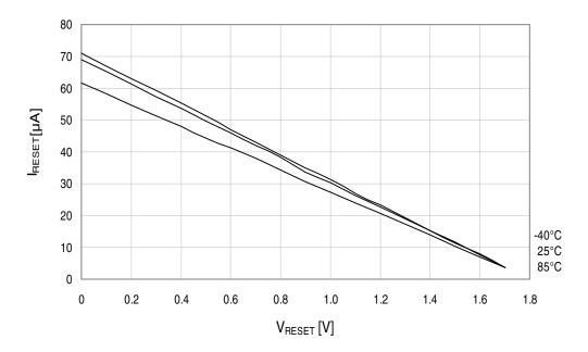
Figure 33-201. Reset pin pull-up resistor current vs. reset pin voltage.  $V_{\rm CC}$  = 3.0V.
