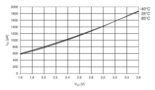
Figure 33-6. Active supply current vs.  $V_{CC}$ .  $f_{SYS} = 32MHz$  internal RC prescaled to 8MHz.
