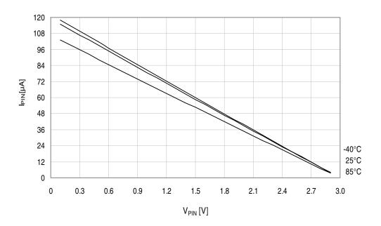
Figure 33-171. I/O pin pull-up resistor current vs. input voltage.  $V_{CC} = 3.3V$ .
