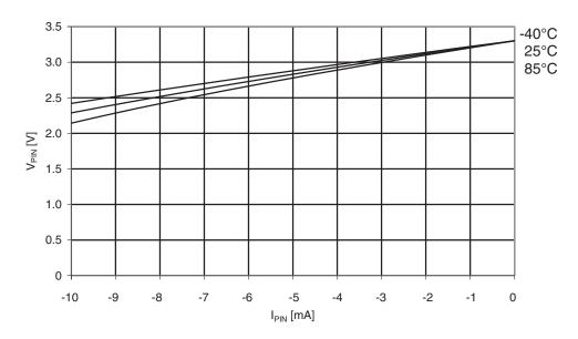
Figure 33-24. I/O pin output voltage vs. sink current.  $V_{CC} = 1.8V$ .
