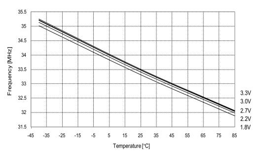
Figure 33-144. 32MHz internal oscillator frequency vs. temperature.
