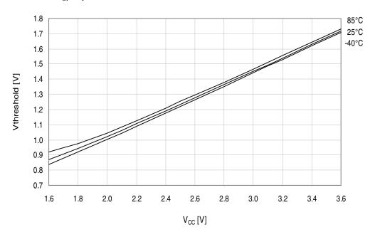
Figure 33-313. I/O pin input threshold voltage vs.  $V_{CC}$ .  $V_{IL}$  I/O pin read as "0".
