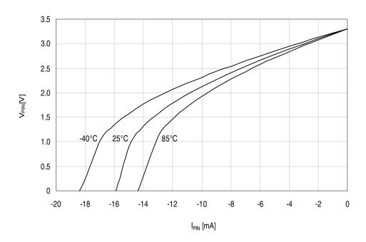
Figure 33-309. I/O pin output voltage vs. sink current.  $V_{CC} = 1.8V$ .
