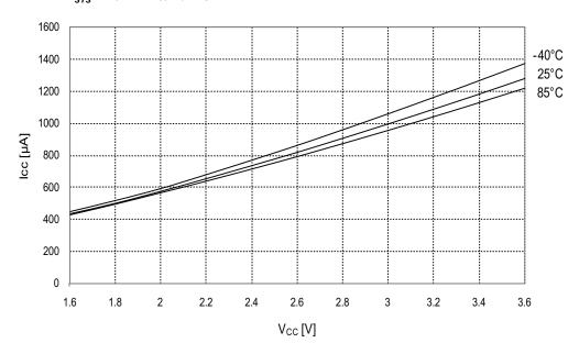
Figure 33-90. Active supply current vs.  $V_{CC}$ .  $f_{SYS} = 32MHz$  internal RC prescaled to 8MHz.
