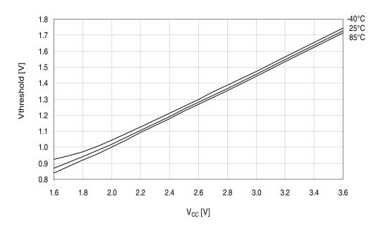
Figure 33-179. I/O pin input threshold voltage vs.  $V_{\rm CC}$ .  $V_{\rm IL}$  I/O pin read as "0".
