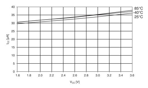
Figure 33-12. Idle supply current vs.  $V_{CC}$ .  $f_{SYS} = 2.0MHz$  internal RC.
