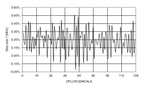
Figure 33-80. Internal 32MHz oscillator CALB calibration step size. T = -40 to 85°C,  $V_{CC} = 3V$ .
