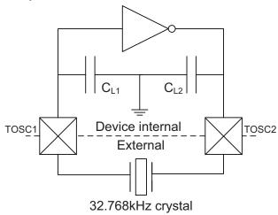
The parasitic capacitance between the TOSC pins is  $C_{L1} + C_{L2}$  in series as seen from the crystal when oscillating without external capacitors.
