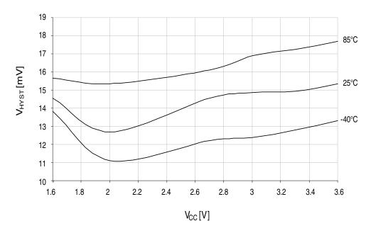
Figure 33-126. Analog comparator hysteresis vs. V<sub>CC</sub>. Large hysteresis.
