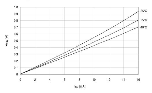
Figure 33-311. I/O pin output voltage vs. sink current.  $V_{CC} = 3.3V$ .
