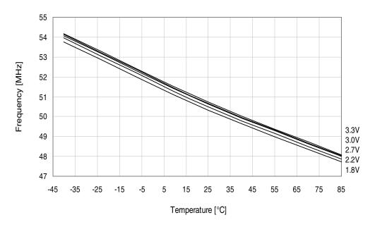
Figure 33-349. 48MHz internal oscillator frequency vs. temperature.
