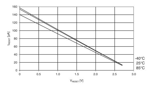
Figure 33-20. Reset pull-up resistor current vs. reset pin voltage.  $V_{CC} = 3.3V$ .
