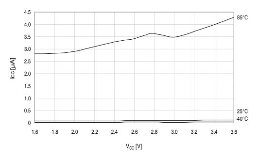
Figure 33-301. Power-down mode supply current vs. V<sub>CC</sub>. Watchdog and sampled BOD enabled.
