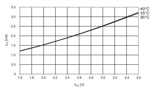
Figure 33-56. Idle supply current vs.  $V_{CC}$ .  $f_{SYS} = 32MHz$  internal RC.
