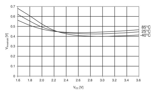
Figure 33-72. Reset input threshold voltage vs.  $V_{CC}$ .  $V_{/L}$  - I/O pin read as "1".
