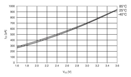
Figure 33-4. Active supply current vs.  $V_{CC}$ .  $f_{SYS} = 32.768kHz$  internal RC.
