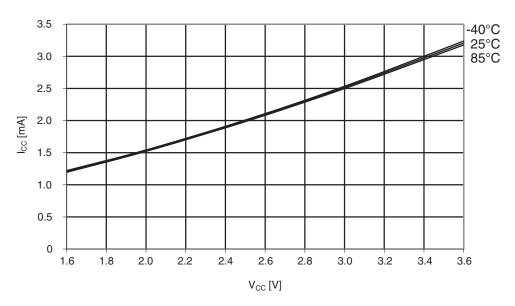
Figure 33-14. Idle supply current vs.  $V_{CC}$ .  $f_{SYS} = 32MHz internal RC$ .
