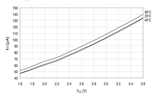
Figure 33-297. Idle mode supply current vs.  $V_{CC}$ .  $f_{SYS} = 2MHz$  internal oscillator.
