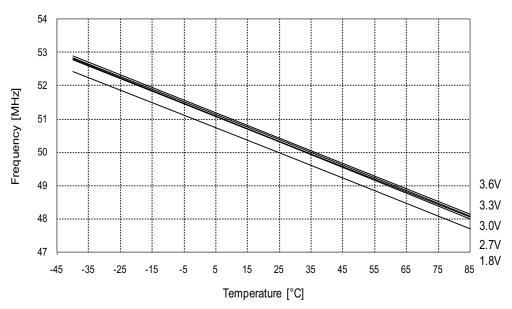
Figure 33-148. 48MHz internal oscillator frequency vs. temperature.
