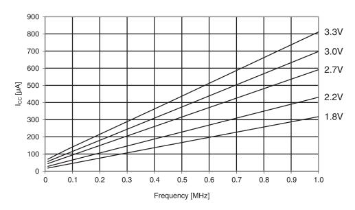
Figure 33-2. Active supply current vs. frequency.  $f_{SYS} = 1 - 32MHz$  external clock,  $T = 25^{\circ}C$ .
