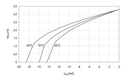
Figure 33-242. I/O pin output voltage vs. sink current.  $V_{CC} = 1.8V$ .
