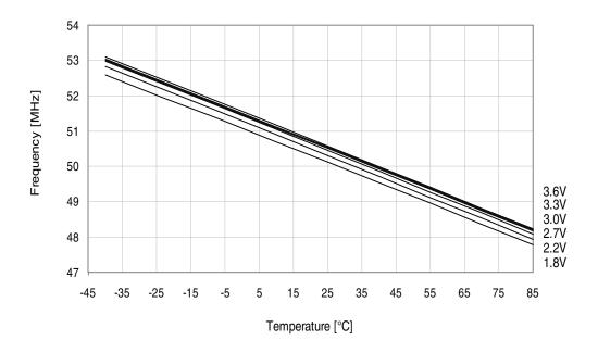
Figure 33-215. 48MHz internal oscillator frequency vs. temperature.
