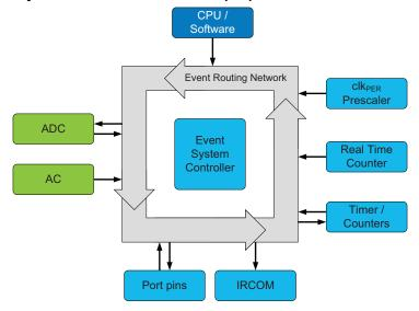
The event routing network consists of four software-configurable multiplexers that control how events are routed and used. These are called event channels, and allow for up to four parallel event routing configurations. The maximum routing latency is two peripheral clock cycles. The event system works in both active mode and idle sleep mode.
