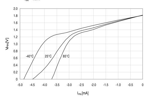
Figure 33-307. I/O pin output voltage vs. source current.  $V_{CC}$  = 3.0V.
