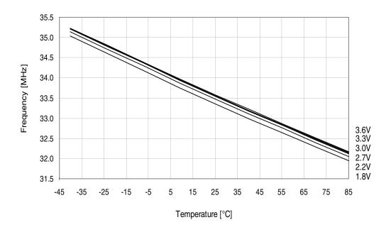
Figure 33-211. 32MHz internal oscillator frequency vs. temperature.
