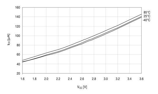
Figure 33-163. Idle mode supply current vs.  $V_{CC}$ .  $f_{SYS} = 2MHz$  internal oscillator.
