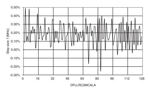
Figure 33-36. Internal 2MHz oscillator CALB calibration step size. T = -40 to 85°C,  $V_{CC} = 3V$ .
