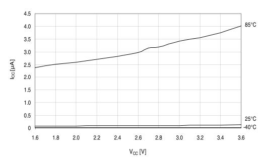
Figure 33-167. Power-down mode supply current vs. V<sub>CC</sub>. Watchdog and sampled BOD enabled.
