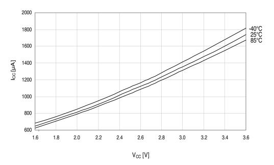
Figure 33-165. Idle mode current vs.  $V_{CC}$ .  $f_{SYS} = 32MHz$  internal oscillator.
