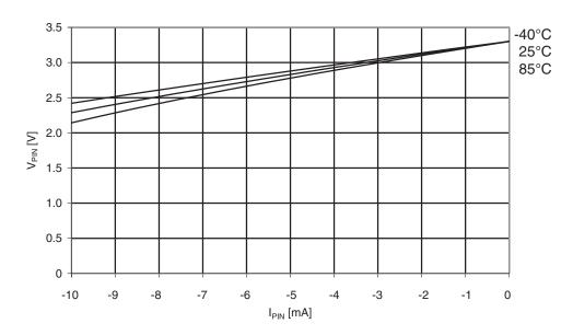
Figure 33-66. I/O pin output voltage vs. sink current.  $V_{CC} = 1.8V$ .
