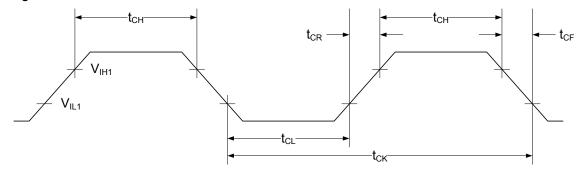
Table 32-53. External clock used as system clock without prescaling.
