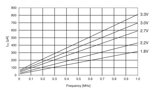
Figure 33-44. Active supply current vs. frequency.  $f_{SYS} = 1 - 32MHz$  external clock,  $T = 25^{\circ}C$ .
