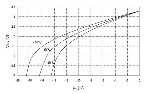
Figure 33-108. I/O pin output voltage vs. sink current.
