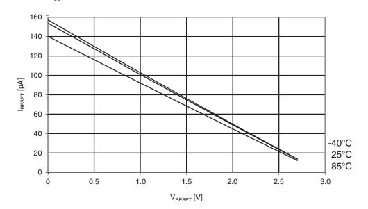
Figure 33-62. Reset pull-up resistor current vs. reset pin voltage.  $V_{cc}$  = 3.3V.
