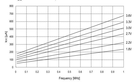
Figure 33-86. Active supply current vs. frequency.  $f_{SYS} = 1 - 32MHz$  external clock,  $T = 25^{\circ}C$ .
