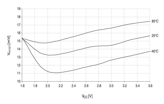
Figure 33-327. Analog comparator hysteresis vs.  $V_{CC}$ . Large hysteresis.
