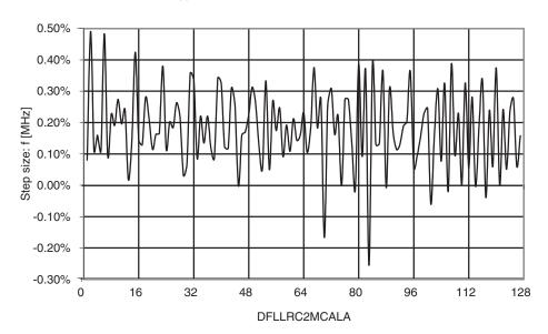
Figure 33-78. Internal 2MHz oscillator CALB calibration step size. T = -40 to 85°C,  $V_{CC} = 3V$ .
