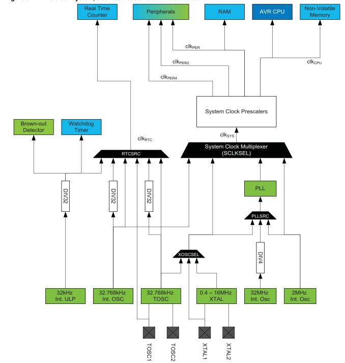
Figure 9-1. The clock system, clock sources and clock distribution.
