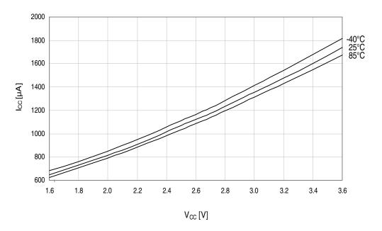
Figure 33-232. Idle mode current vs.  $V_{CC}$ .  $f_{SYS} = 32MHz$  internal oscillator.
