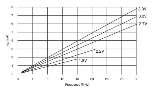
Figure 33-10. Idle supply current vs.  $V_{CC}$ .  $f_{SYS} = 1.0MHz$  external clock.
