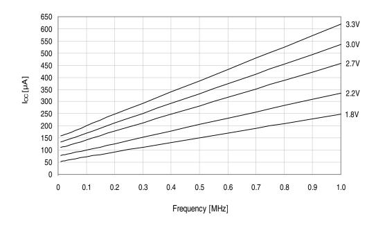
Figure 33-153. Active supply current vs. frequency.  $f_{SYS} = 1 - 32MHz$  external clock,  $T = 25^{\circ}C$ .
