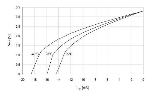
Figure 33-175. I/O pin output voltage vs. sink current.
