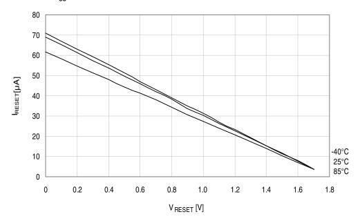
Figure 33-335. Reset pin pull-up resistor current vs. reset pin voltage.  $V_{CC} = 3.0V$ .
