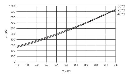
Figure 33-46. Active supply current vs.  $V_{CC}$ .  $f_{SYS} = 32.768kHz$  internal RC.
