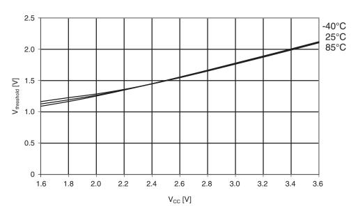
Figure 33-70. I/O pin input threshold voltage vs.  $V_{\rm CC}$ .  $V_{\rm IL}$  - I/O pin read as "0".
