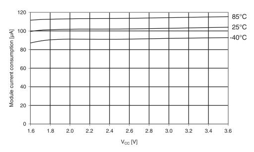
Figure 33-82. Power-up current consumption vs. V<sub>CC</sub>.
