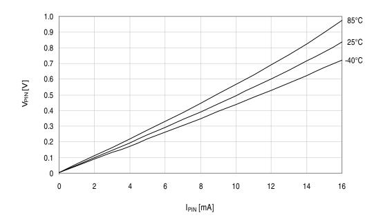
Figure 33-177. I/O pin output voltage vs. sink current.  $V_{CC} = 3.3V$ .
