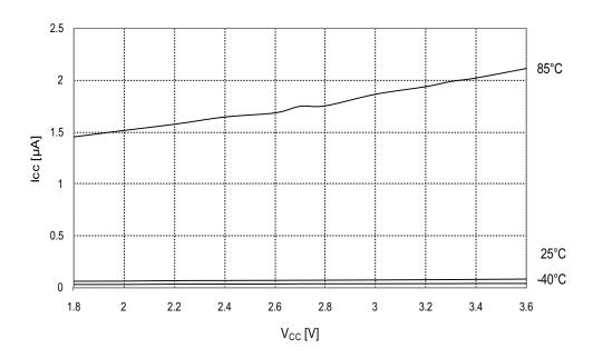
Figure 33-100. Power-down supply current vs.  $V_{\text{CC}}$ . Watchdog and sampled BOD enabled.
