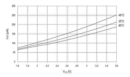
Figure 33-88. Active supply current vs.  $V_{CC}$ .  $f_{SYS} = 1.0MHz$  external clock.
