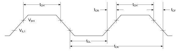
Table 32-110.External clock used as system clock without prescaling.
