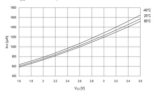
Figure 33-98. Idle supply current vs.  $V_{CC}$ .  $f_{SYS} = 32MHz$  internal RC.
