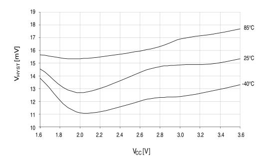
Figure 33-260. Analog comparator hysteresis vs. V<sub>CC</sub>. Large hysteresis.
