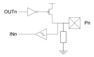
Figure 14-6. I/O configuration - Wired-AND with optional pull-up.
