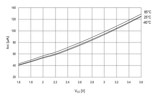
Figure 33-96. Idle supply current vs.  $V_{CC}$ .  $f_{SYS} = 2.0MHz$  internal RC.
