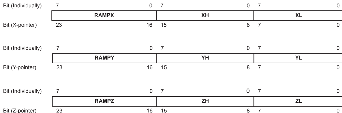
Figure 3-6. The combined RAMPX + X, RAMPY + Y and RAMPZ + Z registers.
