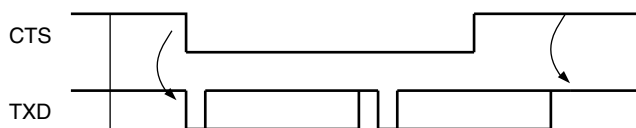
Figure 40-28. Transmitter Behavior when Operating with Hardware Handshaking
