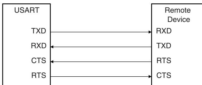
Figure 40-27. Connection with a Remote Device for Hardware Handshaking
