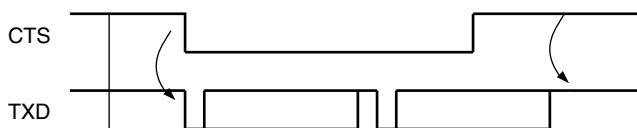
Figure 19-17. Transmitter Behavior when Operating with Hardware Handshaking
