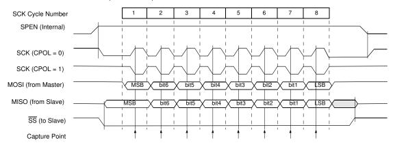
Figure 12. Data Transmission Format (CPHA = 1)
