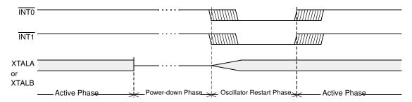
Exiting from power-down by reset redefines all the SFRs, exiting from power-down by external interrupt does no affect the SFRs.
