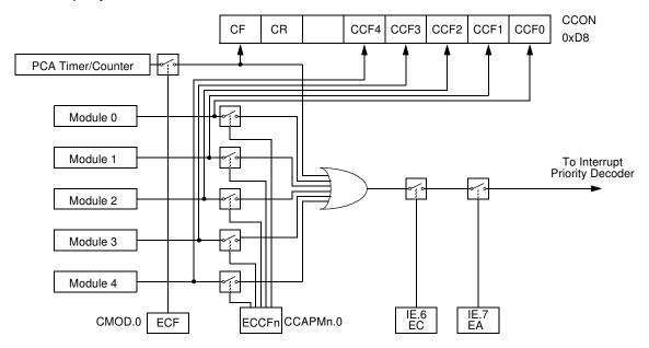
PCA Modules: each one of the five compare/capture modules has six possible functions. It can perform:
