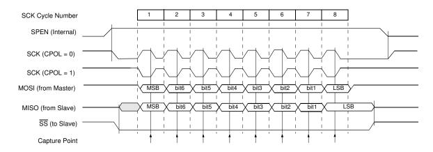
As shown in Figure 11, the first SCK edge is the MSB capture strobe. Therefore, the Slave must begin driving its data before the first SCK edge, and a falling edge on the SS pin is used to start the transmission. The SS pin must be toggled high and then low between each byte transmitted (Figure 13).
