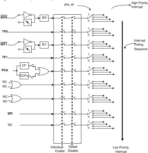
Each of the interrupt sources can be individually enabled or disabled by setting or clearing a bit in the Interrupt Enable register (see Table 31). This register also contains a global disable bit, which must be cleared to disable all interrupts at once.
