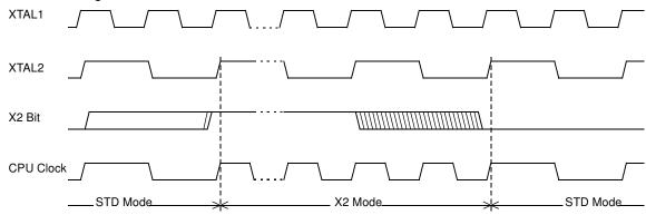
The X2 bit in the CKCON register (See Table 1) allows switching from 12 clock cycles per instruction to 6 clock cycles and vice versa. At reset, the standard speed is activated (STD mode). Setting this bit activates the X2 feature (X2 Mode).
