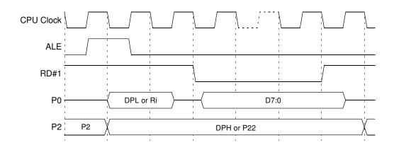
Notes: 1. RD# signal may be stretched using M0 bit in AUXR register.
