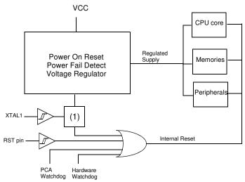
Note: 1. Once XTAL1 high and low levels reach above and below VIH/VIL a 1024 clock period delay will extend the reset coming from the Power Fail Detect. If the power falls below the Power Fail Detect thresthold level, the reset will be applied immediately.
