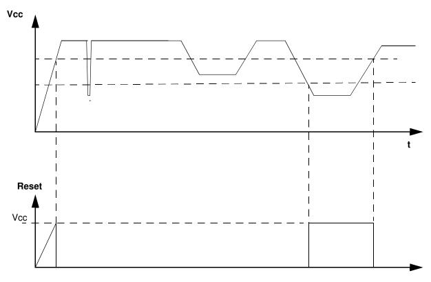
When the power is applied, the Power Monitor immediately asserts a reset. Once the internal supply after the voltage regulator reach a safety level, the power monitor then looks at the XTAL clock input. The internal reset will remain asserted until the Xtal1 levels are above and below VIH and VIL. Further more. An internal counter will count 1024 clock periods before the reset is de-asserted.
