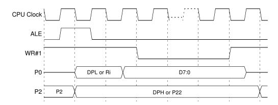
Notes: 1. WR# signal may be stretched using M0 bit in AUXR register.
