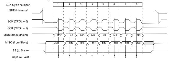
**Figure 47.** Data Transmission Format (CPHA = 1)
