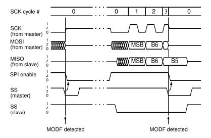
Note: When SS is discarded (SS disabled) it is not possible to detect a MODF error in master mode because the SPI is internally unselected and the SS pin is a general purpose I/O.
