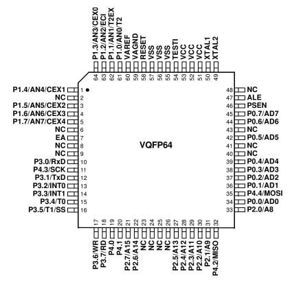
**TESTI** must be connected to VSS
