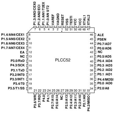
**TESTI** must be connected to VSS
