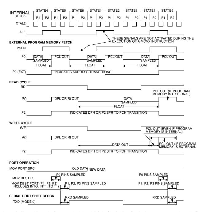
This diagram indicates when signals are clocked internally. The time it takes the signals to propagate to the pins, however, ranges from 25 to 125 ns. This propagation delay is dependent on variables such as temperature and pin loading. Propagation also varies from output to output and component. Typically though ( $T_A$ =25°C fully loaded) RD and WR propagation delays are approximately 50ns. The other signals are typically 85 ns. Propagation delays are incorporated in the AC specifications.
