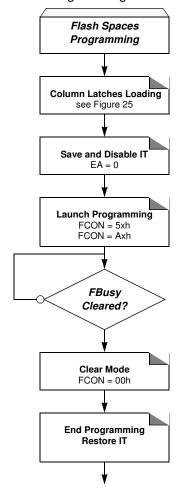
Figure 26. Flash and Extra Row Programming Procedure
