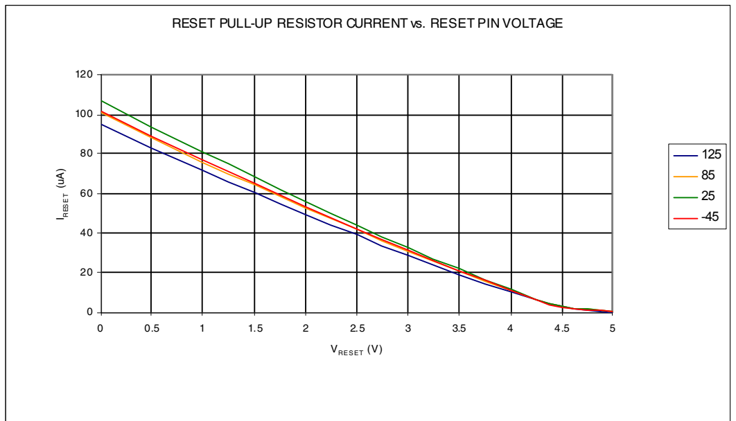
Figure 29-6. Reset Pull-up Resistor Current vs. Reset Pin Voltage ( V_{CC} = 5V ).
