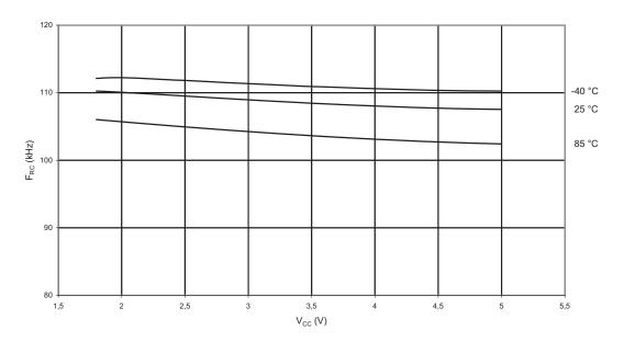
Figure 21-49. Frequency of Watchdog Oscillator vs. Temperature
