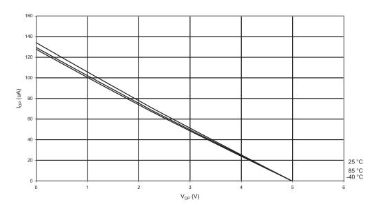
Figure 21-22. Reset Pull-up Resistor Current vs. Reset Pin Voltage (V<sub>CC</sub> = 1.8V) RESET PULL-UP RESISTOR CURRENT vs. RESET PIN VOLTAGE
