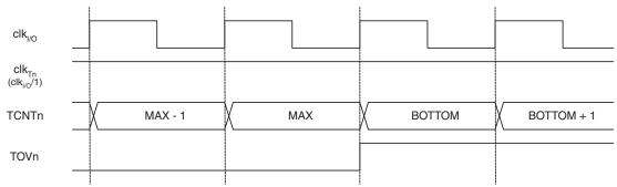
Figure 12-8. Timer/Counter Timing Diagram, no Prescaling
