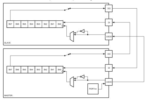
Figure 14-2. Three-wire Mode Operation, Simplified Diagram
