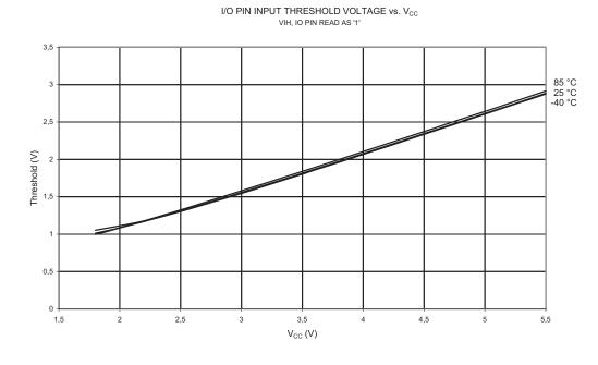
Figure 21-33.  $V_{\text{IH}}$ : Input Threshold Voltage vs.  $V_{\text{CC}}$  (I/O Pin Read as '1')
