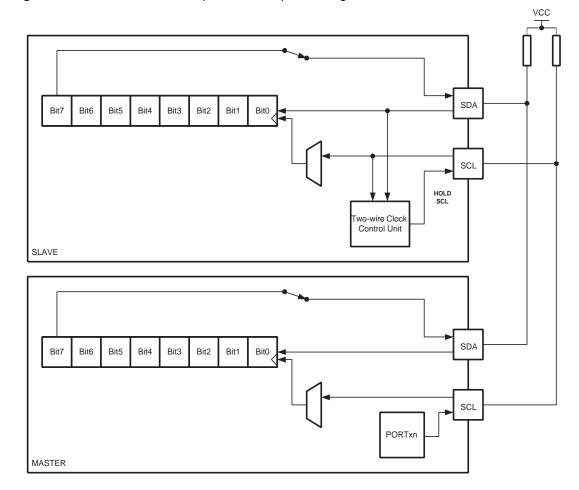
Figure 14-4. Two-wire Mode Operation, Simplified Diagram
