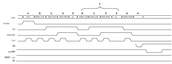
Figure 19-3. Programming the Flash Waveforms <sup>(1)</sup>
