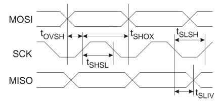
Figure 20-9. Serial Programming Waveforms
