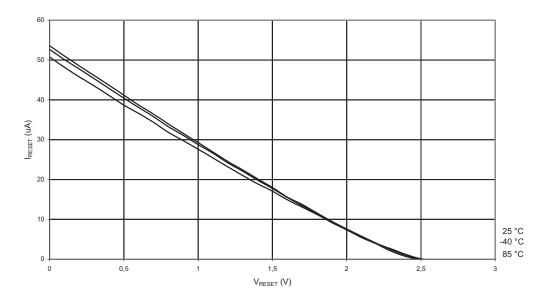
RESET PULL-UP RESISTOR CURRENT vs. RESET PIN VOLTAGE
