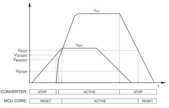
When input voltage  $V_{BAT}$  falls below  $V_{STOP}$  the converter enters Stop Mode and output voltage  $V_{CC}$  begins to fall. When converter output voltage, i.e. the supply voltage of the microcontroller, falls below  $V_{POT}$  the MCU will go into reset.
