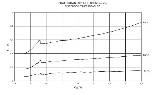
Figure 21-13. Power-down Supply Current vs. V<sub>CC</sub> (Watchdog Timer Disabled)
