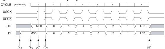
Figure 14-3. Three-wire Mode, Timing Diagram
