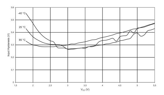
I/O PIN INPUT HYSTERESIS vs. V<sub>CC</sub>
