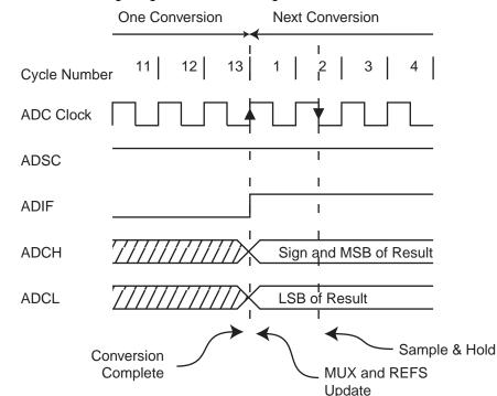
Figure 16-7. ADC Timing Diagram, Free Running Conversion
