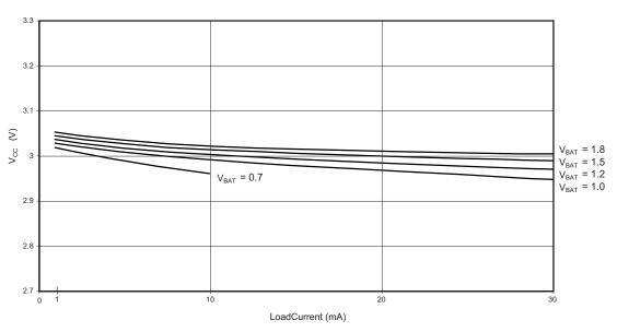
TYPICAL BOOST CONVERTER Vcc vs. LOAD CURRENT
