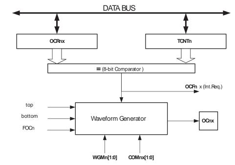
Figure 12-3. Output Compare Unit, Block Diagram
