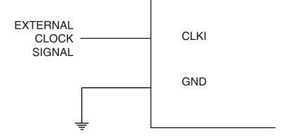
When this clock source is selected, start-up times are determined by SUT Fuses as shown in Table 6-3.
