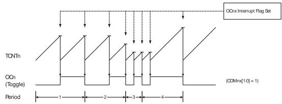
Figure 12-5. CTC Mode, Timing Diagram
