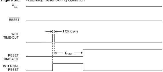
Figure 9-6. Watchdog Reset During Operation
