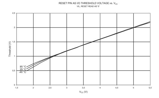
Figure 21-37.  $V_{IL}$ : Input Threshold Voltage vs.  $V_{CC}$  (Reset Pin as I/O, Read as '0')
