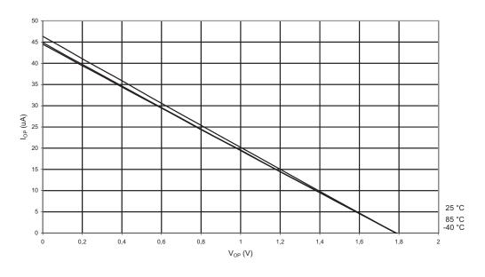
Figure 21-19. Pull-up Resistor Current vs. Input Voltage (I/O Pin,  $V_{CC} = 1.8V$ )
