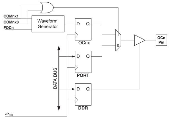
Figure 12-4. Compare Match Output Unit, Schematic (non-PWM Mode)
