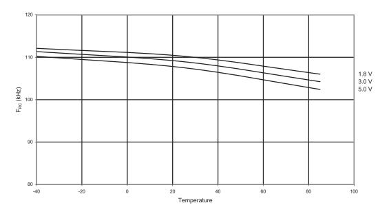
WATCHDOG OSCILLATOR FREQUENCY vs. TEMPERATURE
