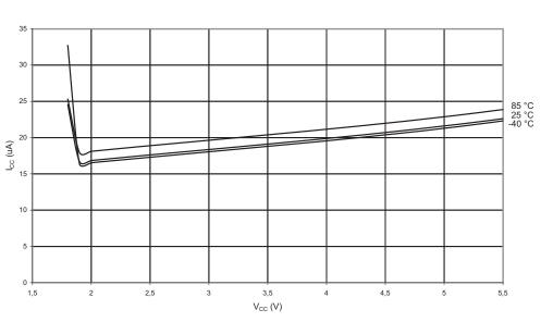
BROWNOUT DETECTOR CURRENT vs. V<sub>CC</sub>
