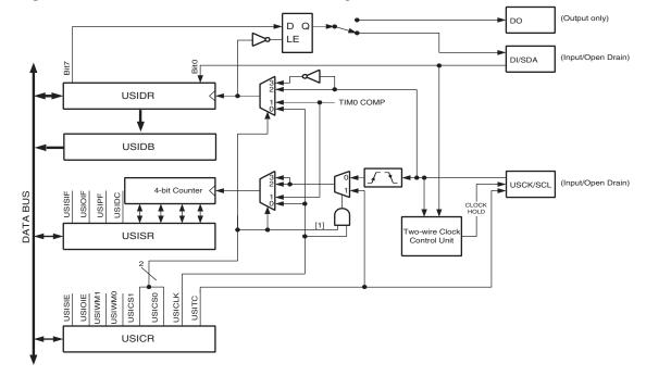
Figure 14-1. Universal Serial Interface, Block Diagram
