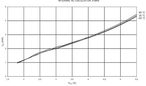
Figure 21-5. Active Supply Current vs. V<sub>CC</sub> (Internal RC Oscillator, 8 MHz) ACTIVE SUPPLY CURRENT vs. V<sub>cc</sub> INTERNAL RC OSCILLATOR, 8 MHz
