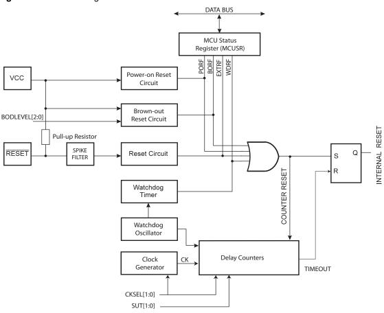
Figure 9-1. Reset Logic
