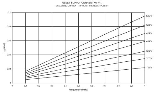
Figure 21-16. Reset Supply Current vs. V<sub>CC</sub> (1 - 20 MHz, Excluding Current Through The Reset Pull-up)
