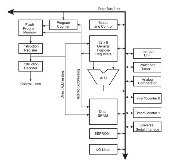
Figure 4-1. Block Diagram of the AVR Architecture
