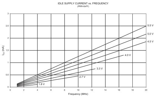
Figure 21-9. Idle Supply Current vs. Frequency (1 - 20 MHz)
