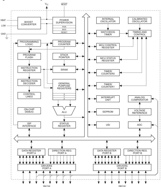
Figure 2-1. Block Diagram
