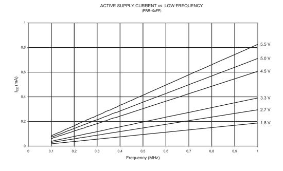
Figure 21-3. Active Supply Current vs. Low Frequency (0.1 - 1.0 MHz)
