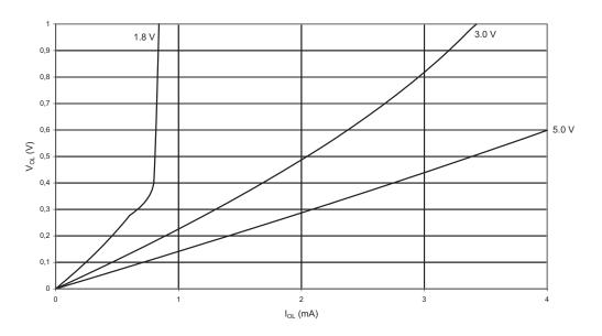
RESET AS I/O PIN OUTPUT VOLTAGE vs. SINK CURRENT
