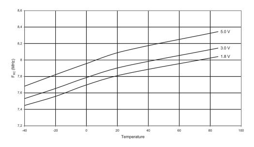
CALIBRATED 8.0MHz RC OSCILLATOR FREQUENCY vs. TEMPERATURE
