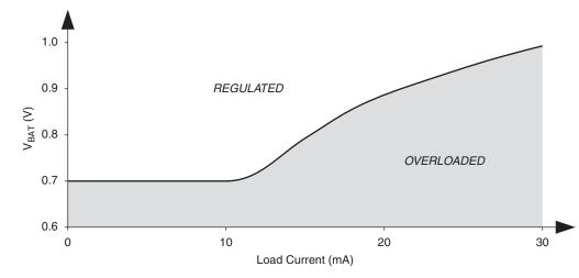
Figure 20-3. Typical V<sub>BAT</sub> Voltage vs. Load Current Required To Maintain Output Regulation.
