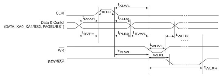
Figure 20-5. Parallel Programming Timing, Including some General Timing Requirements
