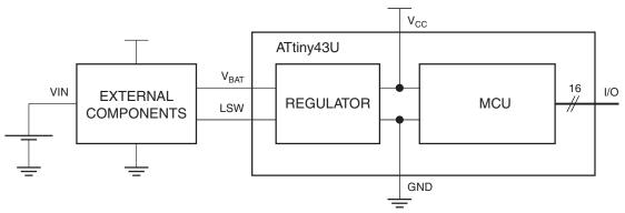
Figure 8-1. Block Diagram of Boost Converter Usage.
