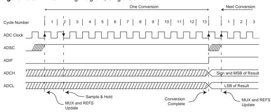
Figure 16-5. ADC Timing Diagram, Single Conversion
