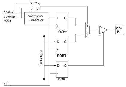
Figure 20-4. Compare Match Output Unit, Schematic
