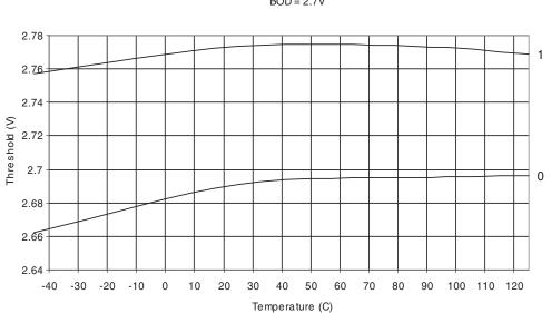
BANDGAP VOLTAGE vs. TEMPERATURE BOD = 2.7V
