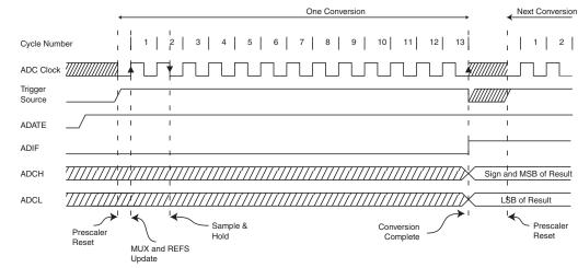
Figure 25-6. ADC Timing Diagram, Auto Triggered Conversion
