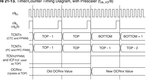
Figure 21-13. Timer/Counter Timing Diagram, with Prescaler ( $f_{clk\_l/O}/8$ )
