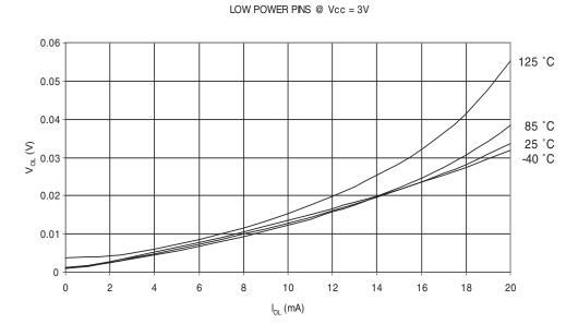
VO PIN OUTPUT VOLTAGE vs. SINK CURRENT
