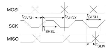
Figure 29-4. Serial Programming Waveforms
