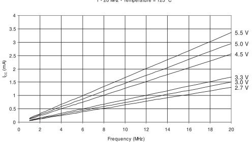
IDLE SUPPLY CURRENT vs. FREQUENCY 1 - 20 MHz - Temperature = 125 °C
