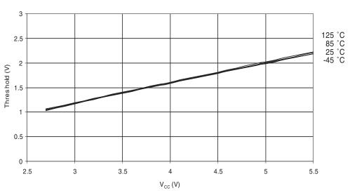
RESET PIN AS 1/O THRESHOLD VOLTAGE vs. V  $_{\rm CC}$  VL, RESET READ AS '0'
