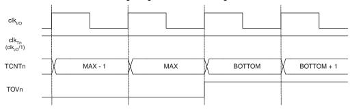
Figure 20-8. Timer/Counter Timing Diagram, no Prescaling
