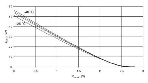
RESET PULL-UP RESISTOR CURRENT vs. RESET PIN VOLTAGE Vcc = 2.7V
