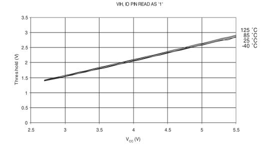
VO PIN INPUT THRESHOLD VOLTAGE vs. Vc
