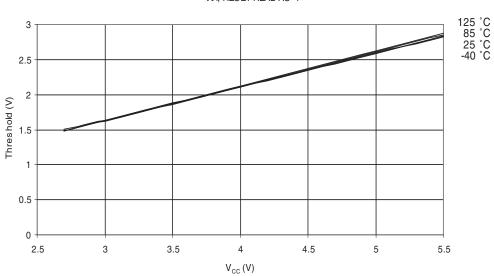
RESET PIN AS 1/O THRESHOLD VOLTAGE vs.  $V_{CC}$  VH, RESET READ AS '1'
