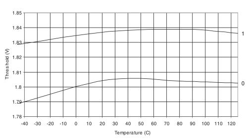
BANDGAP VOLTAGE vs. TEMPERATURE BOD = 1.8V
