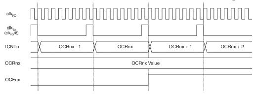
Figure 20-11 on page 99 shows the setting of OCF0A and the clearing of TCNT0 in CTC mode and fast PWM mode where OCR0A is TOP.
