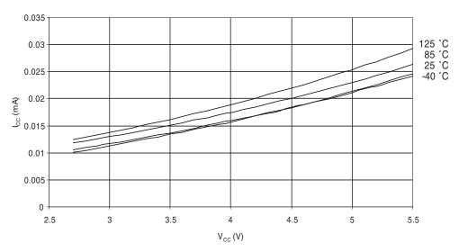
IDLE SUPPLY CURRENT vs.  $V_{\mbox{CC}}$  NTERNAL RC OSCILLATOR, 128 KHz
