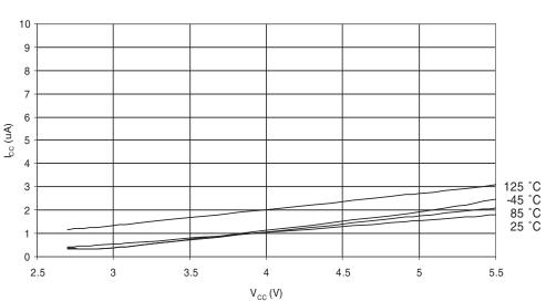
POWER-DOWN SUPPLY CURRENT vs. V<sub>CC</sub> WATCHDOG TIMER ENABLED
