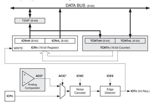
Figure 21-3. Input Capture Unit Block Diagram
