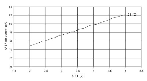
AREF CURRENT vs. AREF VOLTAGE WHEN USED AS ADC REFERENCE  $(\ensuremath{\mathsf{Vcc}=\!5.5V})$
