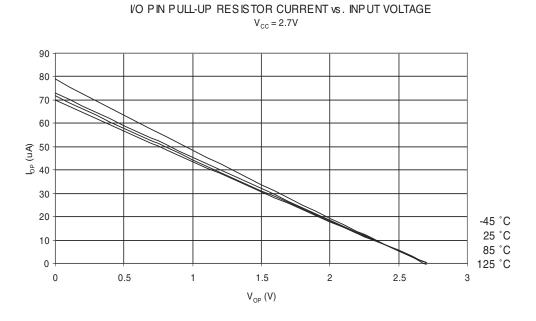
Figure 30-15. I/O Pin Pull-up Resistor Current vs. input Voltage (V<sub>CC</sub> = 2.7V)
