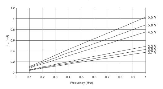
ACTIVE SUPPLY CURRENT vs. LOW FREQUENCY 0.1 - 1.0 MHz - Temperature = 125°C
