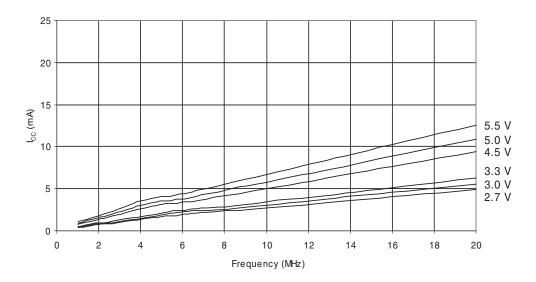
Figure 30-5. Active Supply Current vs. V<sub>CC</sub> (Internal RC Oscillator, 8 MHz)
