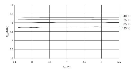
Figure 30-34. Calibrated 8 MHz RC oscillator Frequency vs. Temperature
