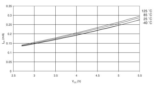
IDLE SUPPLY CURRENT vs. V<sub>CC</sub> NTERNAL RC OSCILLATOR, 1 MHz
