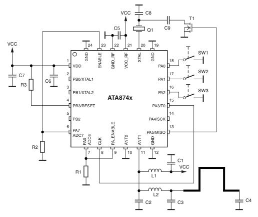
Note: FSK Modulation is achieved by switching on and off an additional capacitor between the XTAL load capacitor and GND. This is done using a MOS switch controlled by a microcontroller output.
