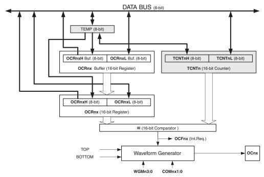
Figure 21-4. Output Compare Unit, Block Diagram
