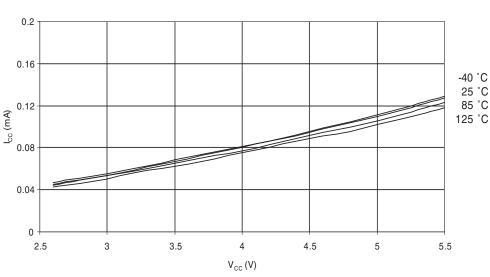
ACTIVE SUPPLY CURRENT vs. V<sub>CC</sub> NTERNAL RC OSCILLATOR, 128 KHz
