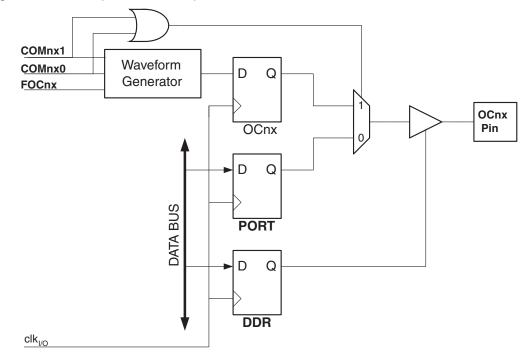
Figure 21-5. Compare Match Output Unit, Schematic
