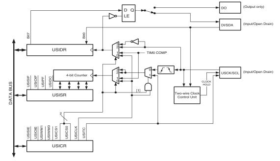
Figure 23-1. Universal Serial Interface, Block Diagram
