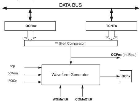
Figure 20-3. Output Compare Unit, Block Diagram
