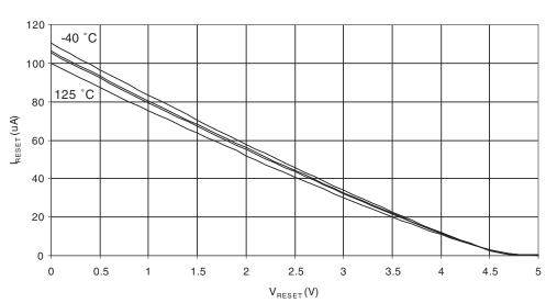
RESET PULL-UP RESISTOR CURRENT vs. RESET PIN VOLTAGE Vcc = 5.0V
