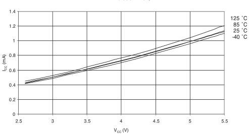
ACTIVE SUPPLY CURRENT vs. V<sub>CC</sub> INTERNAL RC OSCILLATOR, 1MHz
