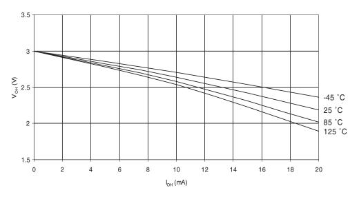
VO PIN OUTPUT VOLTAGE vs. SOURCE CURRENT LOW POWER PNS @ vcc = 3V
