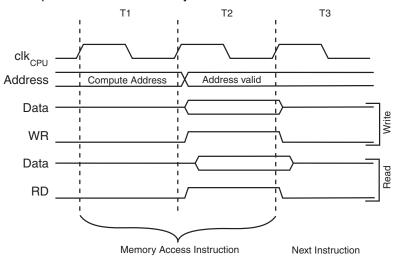
Figure 13-3. On-chip Data SRAM Access Cycles
