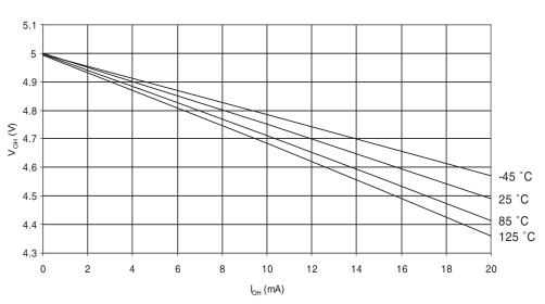
VO PIN OUTPUT VOLTAGE vs. SOURCE CURRENT LOW POWER PINS @ vcc = 5V
