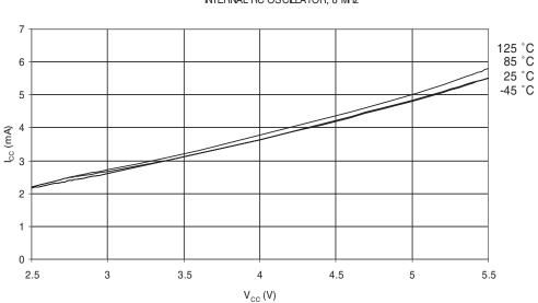
ACTIVE SUPPLY CURRENT vs. V<sub>CC</sub> INTERNAL RC OSCILLATOR, 8 MHz
