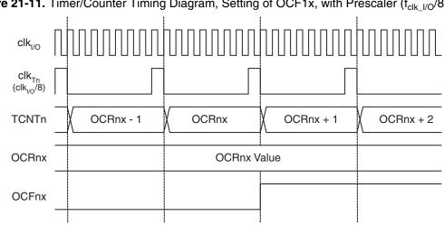
Figure 21-11. Timer/Counter Timing Diagram, Setting of OCF1x, with Prescaler (f<sub>clk I/O</sub>/8)
