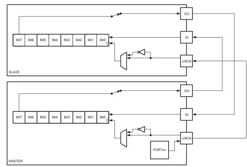
Figure 23-2. Three-wire Mode Operation, Simplified Diagram
