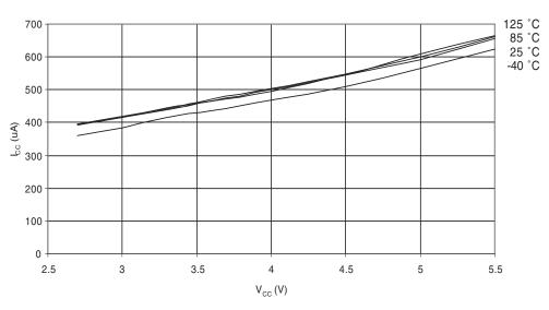
ADC CURRENT vs. Vc 4.0 MHZ FREQUENCY
