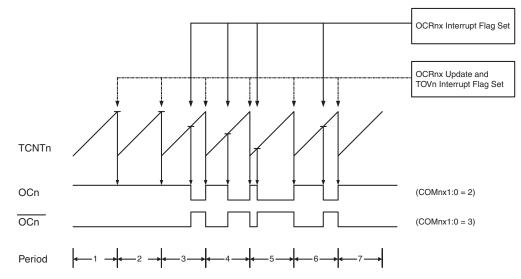
Figure 20-6. Fast PWM Mode, Timing Diagram
