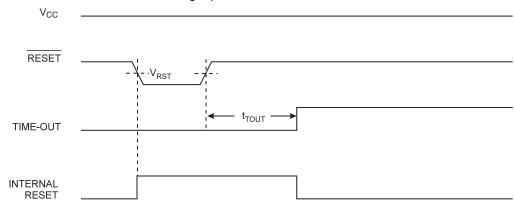
Figure 16-4. External Reset During Operation
