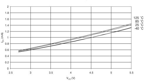
IDLE SUPPLY CURRENT vs. V<sub>CC</sub> NTERNAL RC OSCILLATOR, 8 MHz
