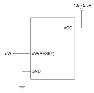
Figure 26-1 on page 173 shows the schematic of a target MCU, with debugWIRE enabled, and the emulator connector. The system clock is not affected by debugWIRE and will always be the clock source selected by the CKSEL Fuses.
