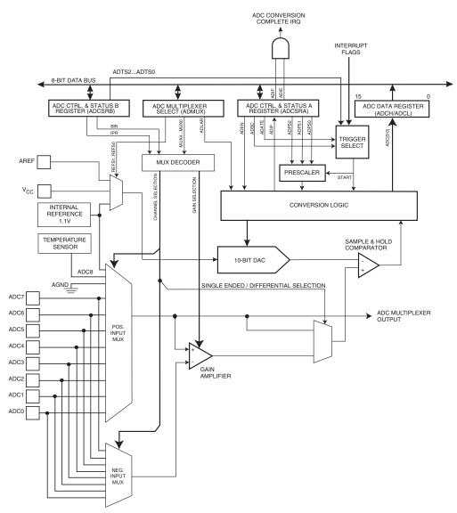
Figure 25-1. Analog to Digital Converter Block Schematic
