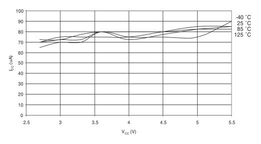
Figure 30-39. Programming Current vs. V<sub>CC</sub>
