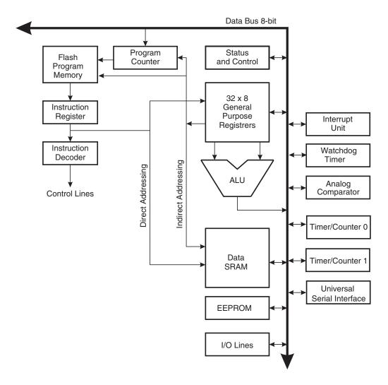
Figure 12-1. Block Diagram of the AVR Architecture
