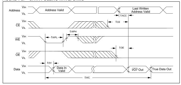
FIGURE 1-4: CHIP CLEAR WAVEFORMS
