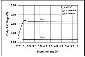
FIGURE 2-4: Output Voltage vs. Input Voltage.
