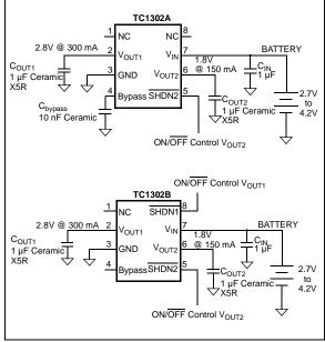
**FIGURE 6-1:** Typical Application Circuit TC1302A/B.
