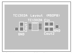
FIGURE 7-1: MSOP8 Silk-screen Layer.
