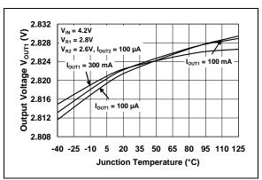
**FIGURE 2-12:** V<sub>OUT1</sub> vs. Junction Temperature.
