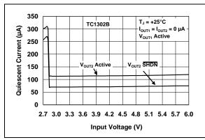
**FIGURE 2-1:** Quiescent Current vs. Input Voltage.
