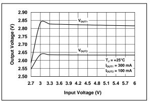
FIGURE 2-5: Output Voltage vs. Input Voltage.
