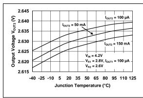
**FIGURE 2-14:** V<sub>OUT2</sub> vs. Junction Temperature.
