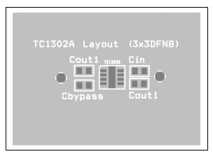
FIGURE 7-2: DFN3x3 Silk-screen Example.
