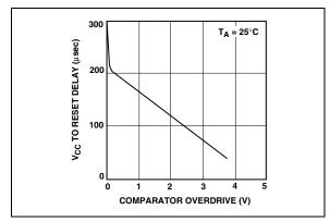
**FIGURE 2-2:** Reset Delays vs. Comparator Overdrive.
