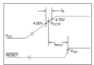
**FIGURE 3-1:** TC1279 Power Up Timing Diagram.
