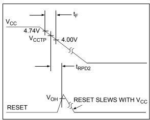
**FIGURE 3-4:** TC1278 Power-Down Timing Diagram.
