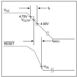
**FIGURE 3-2:** TC1279 Power-Down Timing Diagram.
