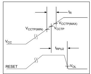
**FIGURE 3-3:** TC1278 Power-Up Timing Diagram.
