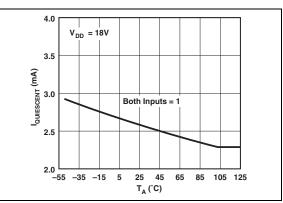
FIGURE 2-11: Supply Current vs. Temperature.
