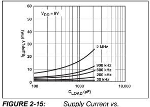
FIGURE 2-15: Capacitive Load.
