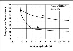
FIGURE 2-7: Propagation Delay Time vs. Input Amplitude.
