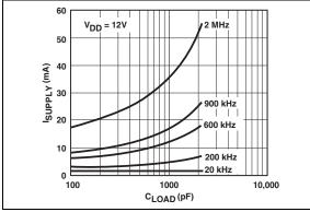
*FIGURE 2-14:* Supply Current vs. Capacitive Load.
