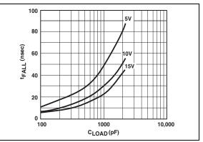
FIGURE 2-5: Fall Time vs. Capacitive Load.
