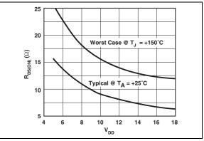
**FIGURE 2-12:** Output Resistance (R<sub>OL</sub>) vs. Supply Voltage.
