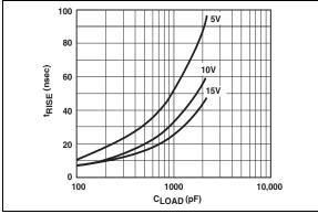
FIGURE 2-2: Rise Time vs. Capacitive Load.
