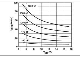
FIGURE 2-1: Rise Time vs. Supply Voltage.
