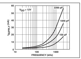
FIGURE 2-17: Supply Current vs. Frequency.
