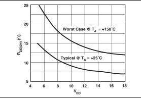
FIGURE 2-9: Supply Voltage.
