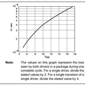
FIGURE 2-19: Crossover Energy vs. Supply Voltage.
