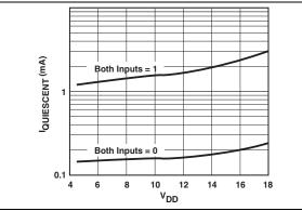
FIGURE 2-8: Supply Current vs. Supply Voltage.
