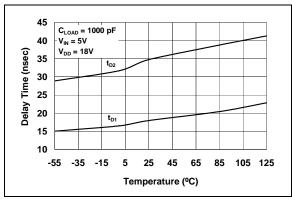
FIGURE 2-10: Propagation Delay Time vs. Temperature.
