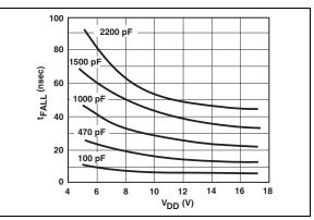
FIGURE 2-4: Fall Time vs. Supply Voltage.
