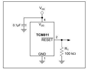
FIGURE 4-2: The addition of  $R_1$  at the RESET output of the TCM811 ensures that the RESET output is valid to  $V_{DD} = 0V$ .
