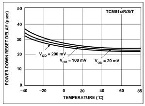
**FIGURE 2-6:** Power-Down Reset Delay vs. Temperature.
