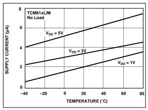
FIGURE 2-4: Supply Current vs. Temperature.
