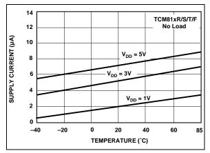
FIGURE 2-1: Supply Current vs. Temperature.
