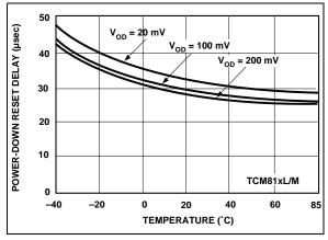
**FIGURE 2-5:** Power-Down Reset Delay vs. Temperature.
