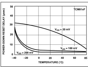
**FIGURE 2-2:** Power-Down Reset Delay vs. Temperature.
