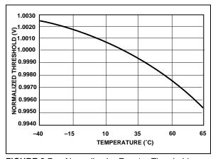
**FIGURE 2-7:** Normalized Reset Threshold vs. Temperature.
