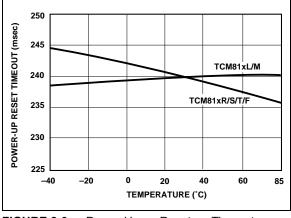
**FIGURE 2-3:** Power-Up Reset Timeout vs. Temperature.
