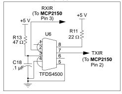
The optical transceiver logic can be implemented with discrete components for cost savings. Care must be taken in the design and layout of the photo detect circuit, due to the small signals that are being detected and their sensitivity to noise. A discrete implementation of the optical transceiver logic is implemented on the DSTEMP and MCP2150 Developer's Kit boards.
