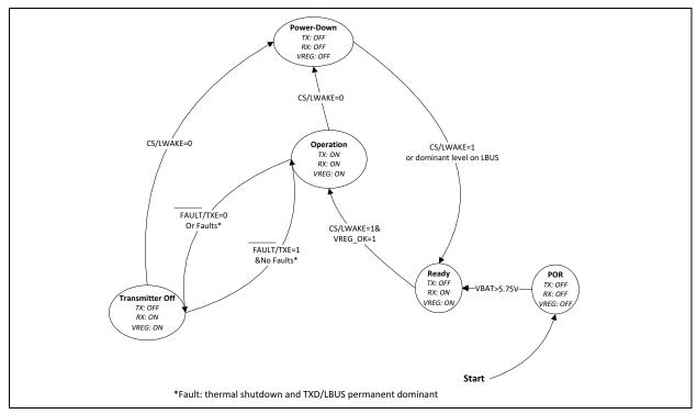
FIGURE 1-2: MCP2021/2 Operational Modes State Diagrams.
