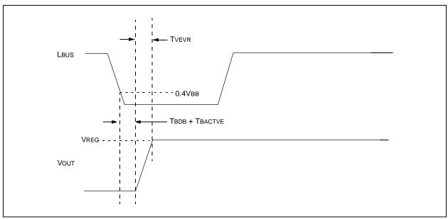
FIGURE 2-6: Regulator BUS WAKE Timing Diagram.
