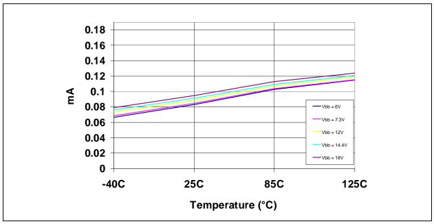
FIGURE 2-10: Typical I<sub>BBTO</sub> vs Temperature.
