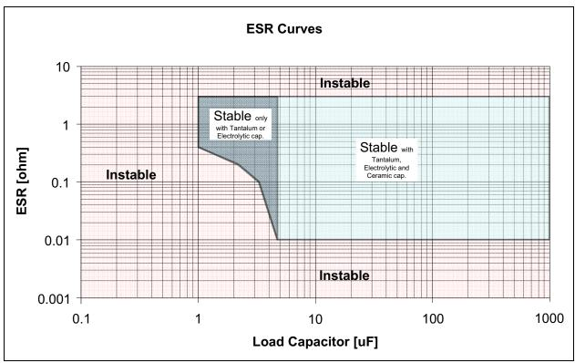
FIGURE 2-3: ESR Curves for Load Capacitor Selection.
