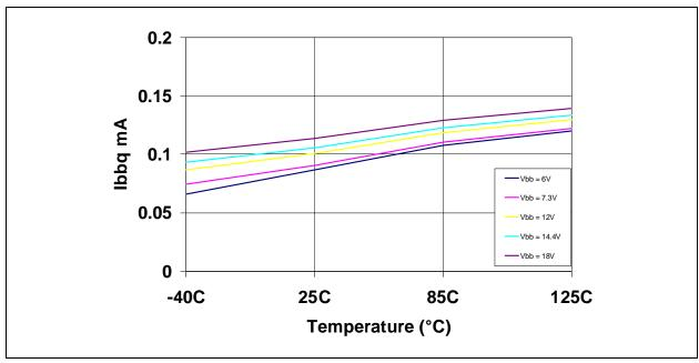
FIGURE 2-9: Typical I<sub>BBQ</sub> vs. Temperature.
