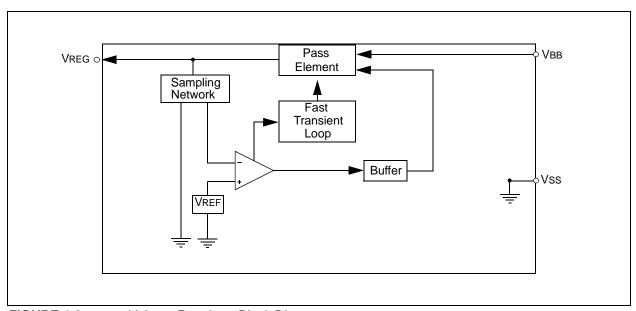
FIGURE 1-9: Voltage Regulator Block Diagram.
