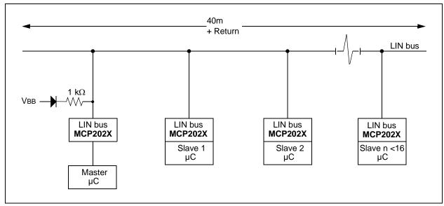
FIGURE 1-8: Typical LIN Network Configuration.
