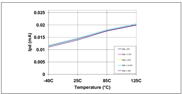
FIGURE 2-11: Typical I<sub>BBPD</sub> vs. Temperature.
