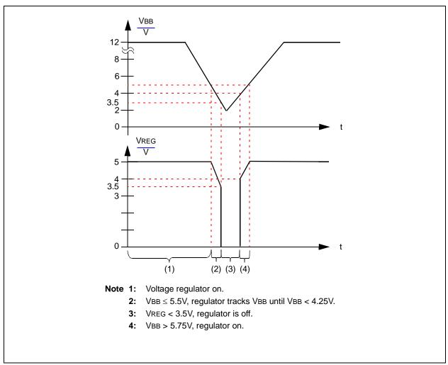
FIGURE 1-11: Voltage Regulator Output on Power Dip.
