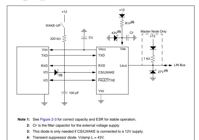
5: These components are required for additional load dump protection above 43V.
