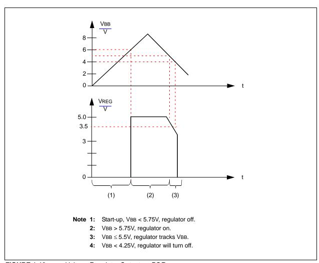
FIGURE 1-10: Voltage Regulator Output on POR.
