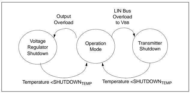
FIGURE 1-1: Thermal Shutdown State Diagrams.
