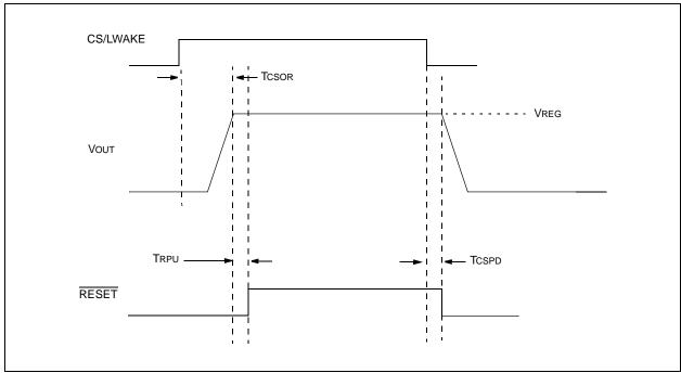
FIGURE 2-8: CS/LWAKE to RESET Timing Diagram.
