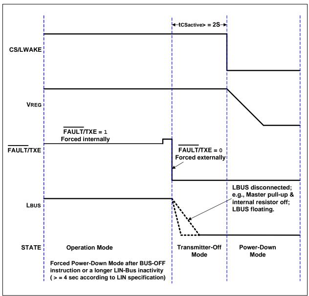
FIGURE 1-5: Forced Power-Down Mode Sequence for MCP2021P/2P.
