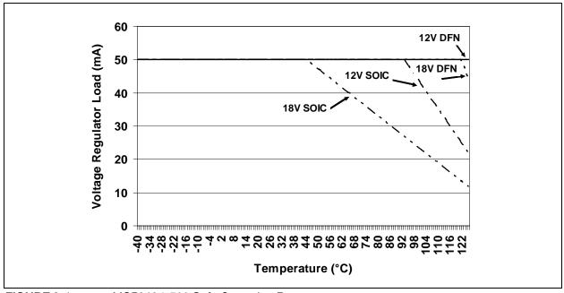
FIGURE 2-1: MCP2021-500 Safe Operating Range.
