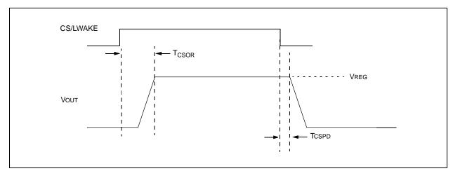
FIGURE 2-5: Regulator CS/LWAKE Timing Diagram.
