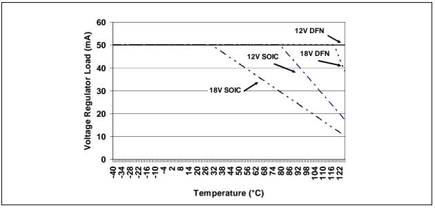
FIGURE 2-2: MCP2021-330 Safe Operating Range.
