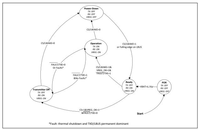
FIGURE 1-3: MCP2021P/2P Operational Modes State Diagrams.
