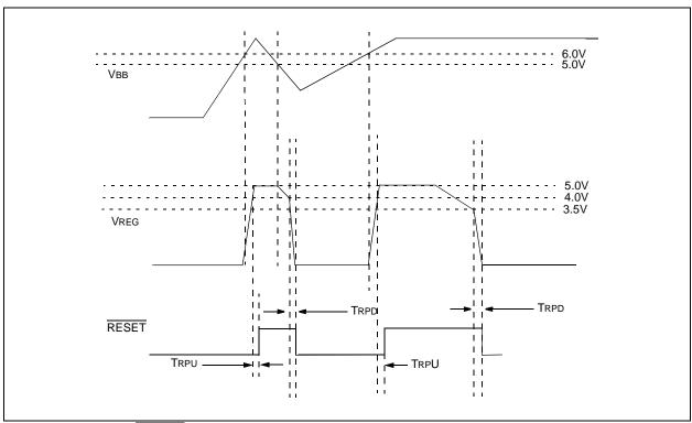
FIGURE 2-7: RESET Timing Diagram.
