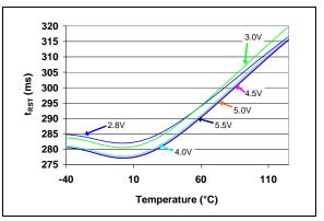
FIGURE 2-30: Reset Time-Out Period (t<sub>RST</sub>) vs. Temperature (TC1270AR, TC1270ANR, TC1271AR - 2.55V min./2.63V typ./2.70V max.).
