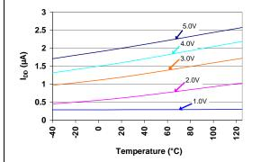
FIGURE 2-2: I<sub>DD</sub> vs. Temperature (Reset Power-up Timer Inactive) (TC1270AT, TC1270ANT, TC1271AT - 3.00V min./3.08V typ./3.15V max.).
