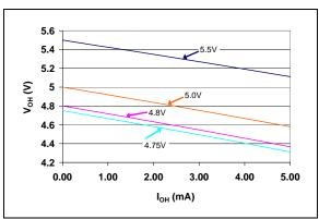
**FIGURE 2-22:** V<sub>OH</sub> vs. I<sub>OL</sub> (TC1270AL, TC1270ANL, TC1271AL - 4.50V min./4.63V typ./4.75V max.) @ +25°C).
