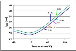
**FIGURE 2-32:** Reset Time-Out Period (t<sub>RST</sub>) (C time out option) vs. Temperature (TC1270AT, TC1270ANT, TC1271AT - 3.00V min./3.08V typ./3.15V max.).
