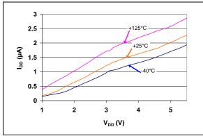
**FIGURE 2-8:** I<sub>DD</sub> vs. V<sub>DD</sub> (Reset Power-up Timer Inactive) (TC1270AT, TC1270ANT, TC1271AT - 3.00V min./3.08V typ./3.15V max.).
