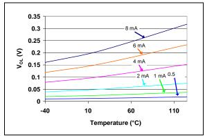
**FIGURE 2-20:** V<sub>OL</sub> vs. Temperature (TC1270AT, TC1270ANT, TC1271AT - 3.00V min./3.08V typ./3.15V max.). @ V<sub>DD</sub> = 2.7V).
