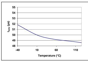
**FIGURE 2-27:** V<sub>DD</sub> Falling to Reset Propagation Delay (t<sub>RPD</sub>) vs. Temperature (TC1270AR, TC1270ANR, TC1271AR - 2.55V min./2.63V typ./2.70V max.).
