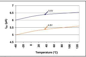
**FIGURE 2-4:** I<sub>DD</sub> vs. Temperature (Reset Power-up Timer Active) (TC1270AL, TC1270ANL, TC1271AL - 4.50V min./4.63V typ./4.75V max.).
