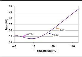
**FIGURE 2-31:** Reset Time-Out Period (t<sub>RST</sub>) (C time out option) vs. Temperature (TC1270AL, TC1270ANL, TC1271AL - 4.50V min./4.63V typ./4.75V max.).
