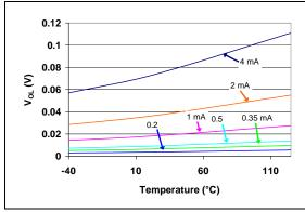
**FIGURE 2-19:** V<sub>OL</sub> vs. Temperature (TC1270AL, TC1270ANL, TC1271AL - 4.50V min./4.63V typ./4.75V max.). @ V<sub>DD</sub> = 4.5V).
