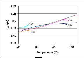
**FIGURE 2-38:** MR Low to Reset Propagation Delay (t<sub>MD</sub>) vs. Temperature (TC1270AT, TC1270ANT, TC1271AT - 3.00V min./3.08V typ./3.15V max.).
