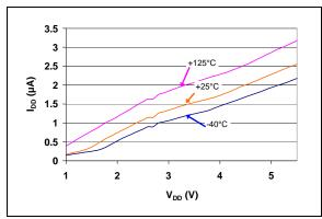
**FIGURE 2-9:** I<sub>DD</sub> vs. V<sub>DD</sub> (Reset Power-up Timer Inactive) (TC1270AR, TC1270ANR, TC1271AR - 2.55V min./2.63V typ./2.70V max.).
