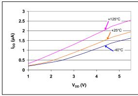
**FIGURE 2-7:** I<sub>DD</sub> vs. V<sub>DD</sub> (Reset Power-up Timer Inactive) (TC1270AL, TC1270ANL, TC1271AL - 4.50V min./4.63V typ./4.75V max.).
