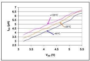
FIGURE 2-11: I<sub>DD</sub> vs. V<sub>DD</sub> (Reset Power-up Timer Active) (TC1270AT, TC1270ANT, TC1271AT - 3.00V min./3.08V typ./3.15V max.).
