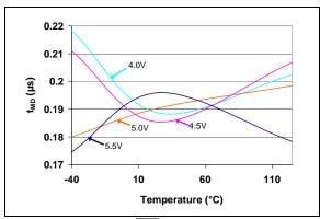
**FIGURE 2-39:** MR Low to Reset Propagation Delay (t<sub>MD</sub>) vs. Temperature (TC1270AR, TC1270ANR, TC1271AR - 2.55V min./2.63V typ./2.70V max.).
