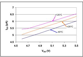
**FIGURE 2-10:** I<sub>DD</sub> vs. V<sub>DD</sub> (Reset Power-up Timer Active) (TC1270AL, TC1270ANL, TC1271AL - 4.50V min./4.63V typ./4.75V max.).
