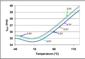
**FIGURE 2-33:** Reset Time-Out Period (t<sub>RST</sub>) (C time out option) vs. Temperature (TC1270AR, TC1270ANR, TC1271AR - 2.55V min./2.63V typ./2.70V max.).
