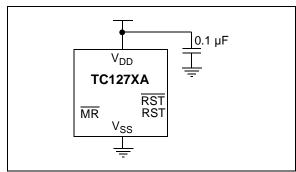
**FIGURE 5-1:** Typical Application Circuit with Bypass Capacitor.
