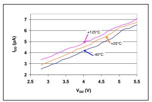
**FIGURE 2-12:** I<sub>DD</sub> vs. V<sub>DD</sub> (Reset Power-up Timer Active) (TC1270AR, TC1270ANR, TC1271AR - 2.55V min./2.63V typ./2.70V max.).
