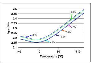
**FIGURE 2-36:** Reset Time-Out Period (t<sub>RST</sub>) (B time out option) vs. Temperature (TC1270AR, TC1270ANR, TC1271AR - 2.55V min./2.63V typ./2.70V max.).
