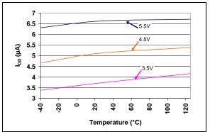
FIGURE 2-5: I<sub>DD</sub> vs. Temperature (Reset Power-up Timer Active) (TC1270AT, TC1270ANT, TC1271AT - 3.00V min./3.08V typ./3.15V max.).
