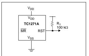
**FIGURE 5-10:** Ensuring a valid active-high Reset pin output state as V<sub>DD</sub> approaches 0V.
