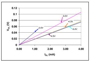
FIGURE 2-16: V<sub>OL</sub> vs. I<sub>OL</sub> (TC1270AL, TC1270ANL, TC1271AL - 4.50V min./4.63V typ./4.75V max.).
