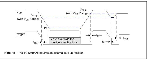
FIGURE 4-8: RST Operation as determined by the V<sub>TRIP</sub>
