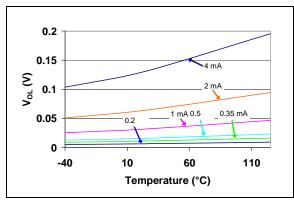
FIGURE 2-21: V<sub>OL</sub> vs. Temperature (TC1270AR, TC1270ANR, TC1271AR - 2.55V min./2.63V typ./2.70V max.). @ V<sub>DD</sub> = 1.8V).
