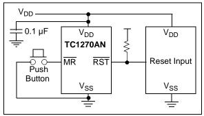
FIGURE 4-3: Typical Open-Drain Application Circuit.
