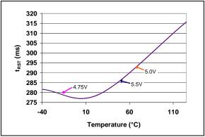
**FIGURE 2-28:** Reset Time-Out Period (t<sub>RST</sub>) vs. Temperature (TC1270AL, TC1270ANL, TC1271AL
