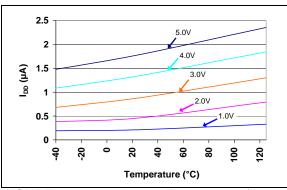
**FIGURE 2-1:** I<sub>DD</sub> vs. Temperature (Reset Power-up Timer Inactive) (TC1270AL, TC1270ANL, TC1271AL - 4.50V min./4.63V typ./4.75V max.).
