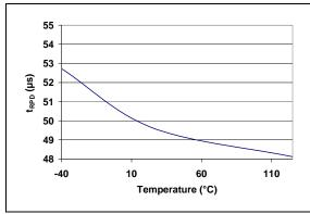
**FIGURE 2-25:** V<sub>DD</sub> Falling to Reset Propagation Delay (t<sub>RPD</sub>) vs. Temperature (TC1270AL, TC1270ANL, TC1271AL - 4.50V min./4.63V typ./4.75V max.).
