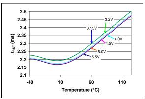
**FIGURE 2-35:** Reset Time-Out Period (t<sub>RST</sub>) (B time out option) vs. Temperature (TC1270AT, TC1270ANT, TC1271AT - 3.00V min./3.08V typ./3.15V max.).
