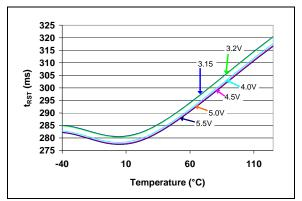
FIGURE 2-29:Reset Time-Out Period  $(t_{RST})$ vs. Temperature
