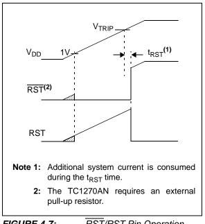
FIGURE 4-7: RST/RST Pin Operation Power-up.
