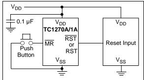
**FIGURE 4-2:** Typical Push-Pull Application Circuit.
