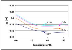
FIGURE 2-37: MR Low to Reset Propagation Delay (t<sub>MD</sub>) vs. Temperature (TC1270AL, TC1270ANL, TC1271AL - 4.50V min./4.63V typ./4.75V max.).
