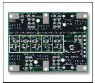
FIGURE 8-1: SOT-23-5/6 Voltage Supervisor Evaluation Board (VSUPEV2).
