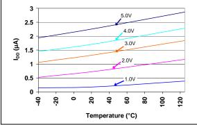
**FIGURE 2-3:** I<sub>DD</sub> vs. Temperature (Reset Power-up Timer Inactive) (TC1270AR, TC1270ANR, TC1271AR - 2.55V min./2.63V typ./2.70V max.).
