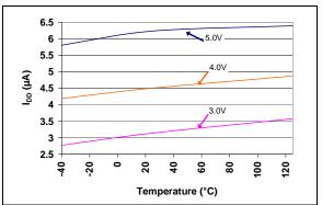
FIGURE 2-6: I<sub>DD</sub> vs. Temperature (Reset Power-up Timer Active) (TC1270AR, TC1270ANR, TC1271AR - 2.55V min./2.63V typ./2.70V max.).
