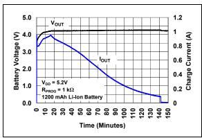
**FIGURE 2-26:** Complete Charge Cycle (1200 mAh Li-lon Battery).
