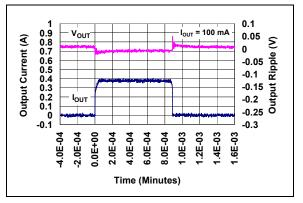
FIGURE 2-22: Load Transient Response.
