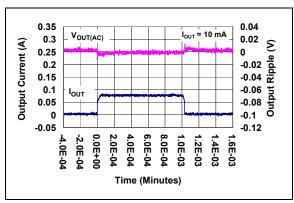
FIGURE 2-21: Load Transient Response.
