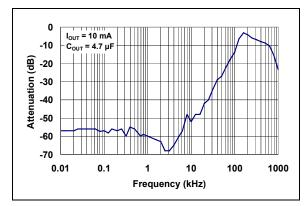
**FIGURE 2-17:** Power Supply Ripple Rejection (PSRR).
