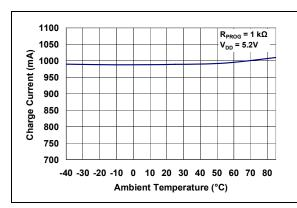
**FIGURE 2-9:** Charge Current ( $I_{OUT}$ ) vs. Ambient Temperature ( $T_A$ ).
