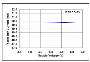
**FIGURE 2-15:** Thermistor Current ( $I_{THERM}$ ) vs. Supply Voltage ( $V_{DD}$ ).
