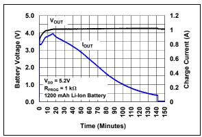
**FIGURE 6-2:** Typical Charge Profile (1200 mAh Li-Ion Battery).
