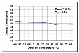
**FIGURE 2-11:** Charge Current ( $I_{OUT}$ ) vs. Ambient Temperature ( $T_{\Delta}$ ).
