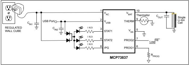
FIGURE 6-1: MCP73837 Typical Stand-Alone Application Circuit.
