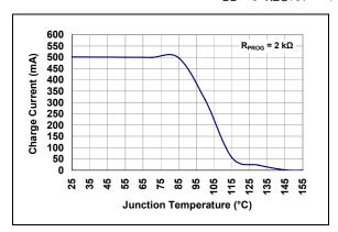
**FIGURE 2-13:** Charge Current ( $I_{OUT}$ ) vs. Junction Temperature ( $T_{II}$ ).
