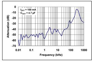
FIGURE 2-18: Power Supply Ripple Rejection (PSRR).
