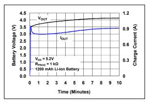
**FIGURE 2-27:** Typical Charge Profile in Thermal Regulation (1200 mAh Li-Ion Battery).
