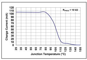
**FIGURE 2-14:** Charge Current  $(I_{OUT})$  vs. Junction Temperature  $(T_1)$ .
