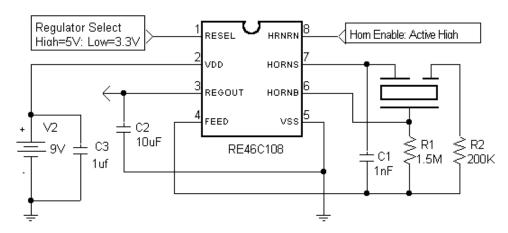
Typical Application Using Self Resonating Piezoelectric Horn
