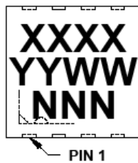
8-Lead DFN (3x3) (MCP622)
