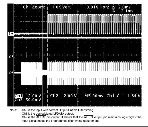
FIGURE 2-16: ALERT Output Example: With No Parity Error and no 32 ms Alarm Timer Time-out.
