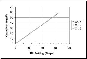
**FIGURE 2-11:** Typical Tuned Capacitance Value vs. Configuration Register Bit Setting  $(V_{DD} = 3V, Temperature = +85^{\circ}C.$
