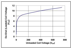
FIGURE 2-6: De-Q-ed Voltage vs. Unloaded Coil Voltage.
