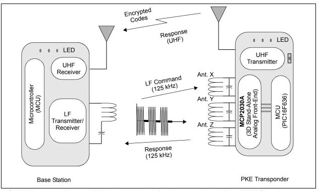
FIGURE 4-3: Example of Bidirectional Hands-free Passive Keyless Entry (PKE) System.
