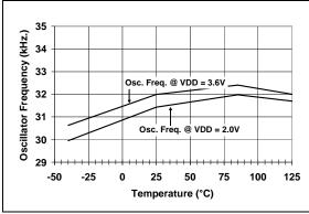
**FIGURE 2-3:** Oscillator Frequency vs. Temperature,  $V_{DD} = 3.6V$  and 2.0V.
