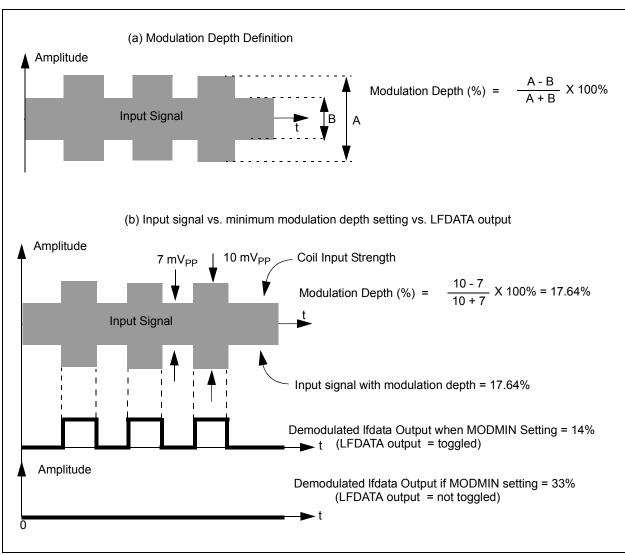
FIGURE 5-5: Modulation Depth Examples.
