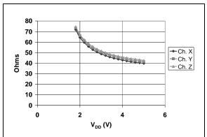
**FIGURE 2-7:** Modulation Transistor-on Resistance (+25°C).
