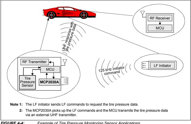
FIGURE 4-4: Example of Tire Pressure Monitoring Sensor Applications.
