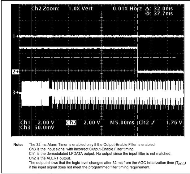
FIGURE 2-17: ALERT Output Example: With 32 ms Alarm Timer Timed-out.
