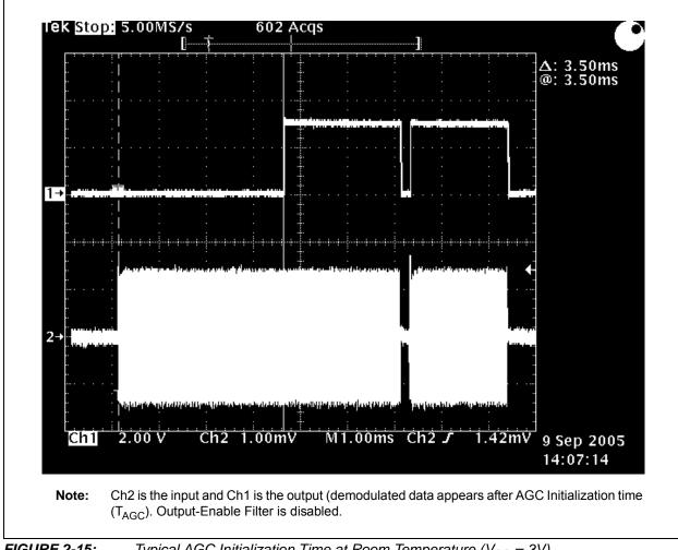
Typical AGC Initialization Time at Room Temperature ( $V_{DD} = 3V$ ). FIGURE 2-15:
