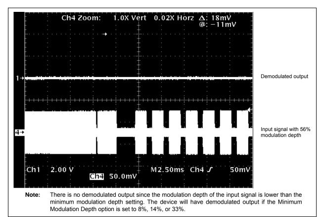
**FIGURE 2-21:** Example of Minimum Modulation Depth Setting: Modulation Depth of Input Signal = 56%, Minimum Modulation Depth (MODMIN) Setting = 60%.
