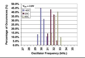
**FIGURE 2-4:** Oscillator Frequency Histograms vs. Temperature,  $V_{DD} = 2V$ .
