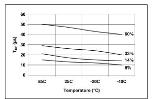
**FIGURE 2-13:** Example of Typical  $T_{DF}$ Changes over Temperature. Input Signal Condition: Amplitude = 300 mVpp, Modulation Depth = 100%.
