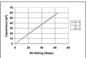
**FIGURE 2-8:** Typical Tuned Capacitance Value vs. Configuration Register Bit Setting  $(V_{DD} = 3V, Temperature = +25^{\circ}C)$ .
