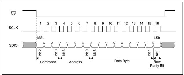
FIGURE 5-12: Detailed SPI Timing (AFE).
