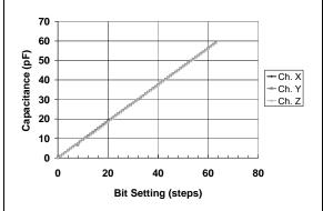
**FIGURE 2-10:** Typical Tuned Capacitance Value vs. Configuration Register Bit Setting  $(V_{DD} = 3V, Temperature = -40^{\circ}C.$
