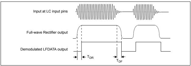
FIGURE 5-6: Demodulator Charge and Discharge.
