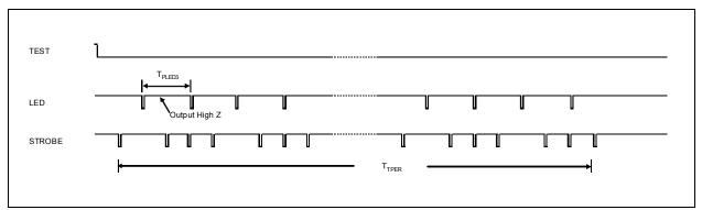
FIGURE 3-3: RE46C165/6/7/8 Timing Diagram – Timer Mode.
