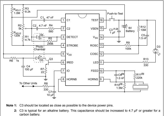
3: R10, R11 and C6 are typical values and may be adjusted to maximize sound pressure.
