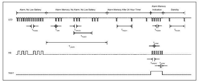
FIGURE 3-4: RE46C165/7 Timer Diagram – Alarm Memory Mode.
