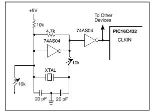
Figure 9-4 shows a series resonant oscillator circuit. This circuit is also designed to use the fundamental frequency of the crystal. The inverter performs a 180° phase shift in a series resonant oscillator circuit. The 330 k $\Omega$  resistors provide the negative feedback to bias the inverters in their linear region.
