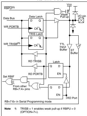
This interrupt can wake the device from SLEEP. The user, in the Interrupt Service Routine, can clear the interrupt in the following manner:
