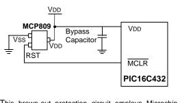
This brown-out protection circuit employs Microchip Technology's MCP809 microcontroller supervisor. The MCP8XX and MCP1XX families of supervisors provide push-pull and open collector outputs with both high and low active RESET pins. There are 7 different trip point selections to accommodate 5V and 3V systems.
