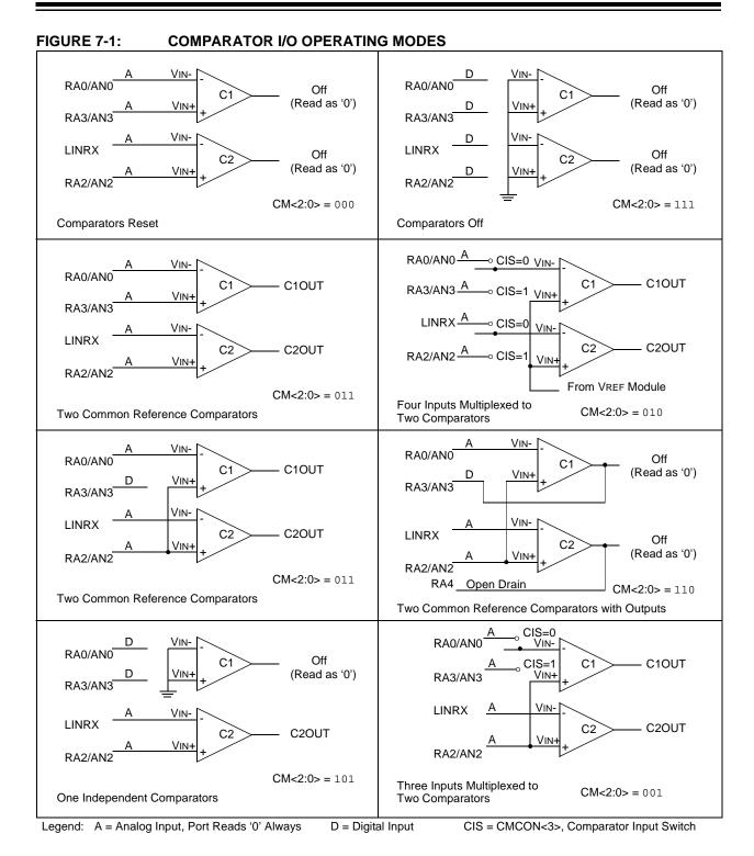
The code example in Example 7-1 depicts the steps required to configure the comparator module. RA3 and RA4 are configured as digital output. RA0 and RA1 are configured as the V- inputs and RA2 as the V+ input to both comparators.
