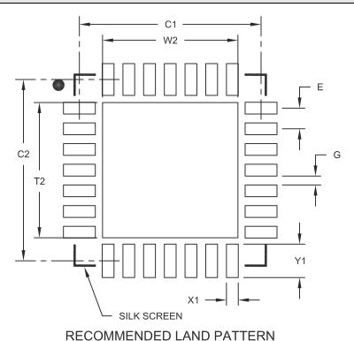
MILLIMETERS Units Dimension Limits NOM MIN MAX Contact Pitch 0.65 BSC Ε Optional Center Pad Width W2 4.25 Optional Center Pad Length T2 4.25 5.70 Contact Pad Spacing C1 Contact Pad Spacing C2 5.70 Contact Pad Width (X28) X1 0.37 Contact Pad Length (X28) Y1 1.00 Distance Between Pads G 0.20
