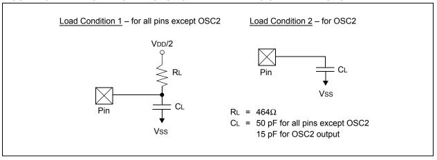
TABLE 28-15: CAPACITIVE LOADING REQUIREMENTS ON OUTPUT PINS
