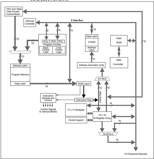
FIGURE 3-2: PIC24HJ32GP302/304, PIC24HJ64GPX02/X04 AND PIC24HJ128GPX02/X04 PROGRAMMER'S MODEL
