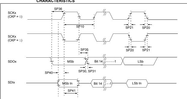
FIGURE 28-11: SPIX MASTER MODE (FULL-DUPLEX, CKE = 1, CKP = x, SMP = 1) TIMING CHARACTERISTICS
