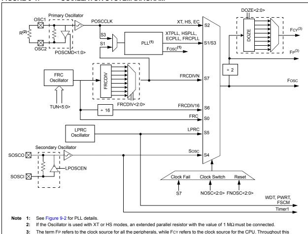
3: The term FP refers to the clock source for all the peripherals, while FcY refers to the clock source for the CPU. Throughout this document FcY and FP are used interchangeably, except in the case of Doze mode. FP and FcY will be different when Doze mode is used in any ratio other than 1:1, which is the default.
