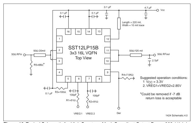
**Figure 10:** Typical Schematic for High Spectrum Mask Compliant Output Power 802.11b/g/n Applications for 16-contact VQFN
