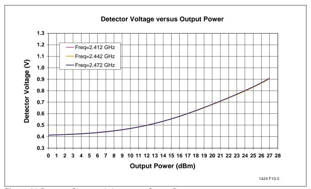
Figure 21: Detector Characteristics versus Output Power
