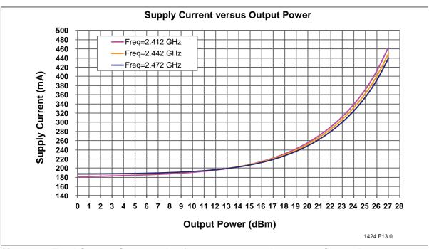
Figure 8: Total Current Consumption for 802.11g operation versus Output Power
