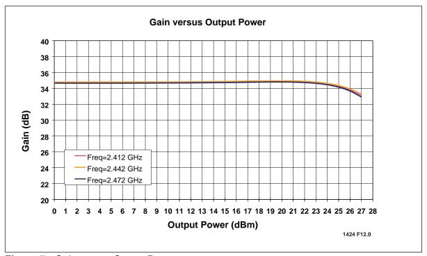
Figure 7: Gain versus Output Power
