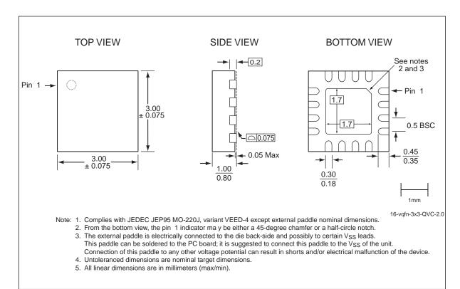
Figure 23:16-contact Very-thin Quad Flat No-lead (VQFN) SST Package Code: QVC
