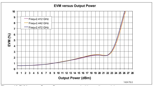
**Figure 18:**EVM versus Output Power measured with equalizer training set to sequence only
