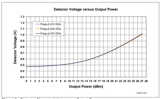
Figure 9: Detector Characteristics versus Output Power
