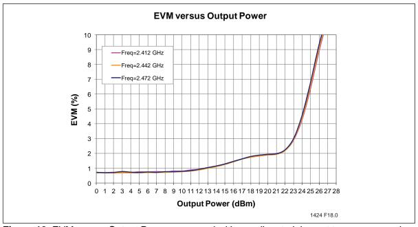
Figure 12: EVM versus Output Power measured with equalizer training set to sequence only
