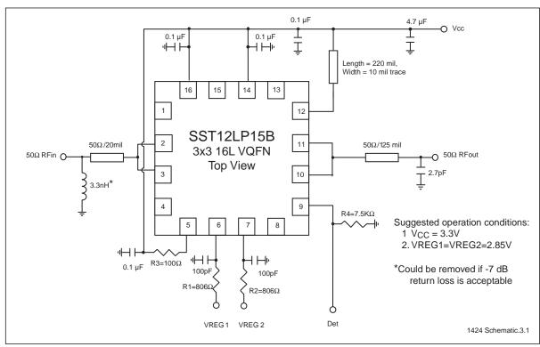
Figure 22: Typical Schematic for High-Linearity 802.11b/g/n Applications for 16-contact VOEN
