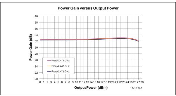
Figure 13: Gain versus Output Power
