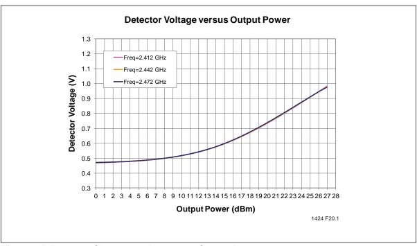
Figure 15: Detector Characteristics versus Output Power
