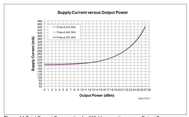
Figure 14: Total Current Consumption for 802.11g operation versus Output Power
