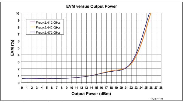
Figure 6: EVM versus Output Power measured with equalizer training set to sequence only
