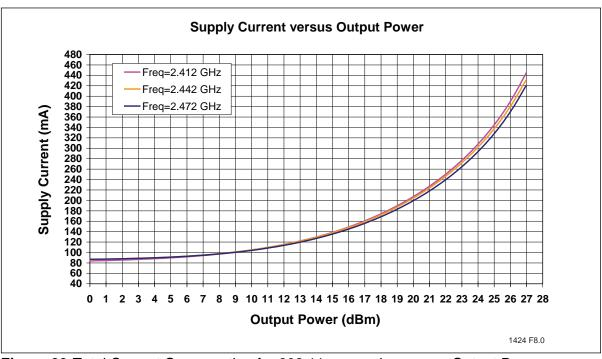
Figure 20: Total Current Consumption for 802.11g operation versus Output Power
