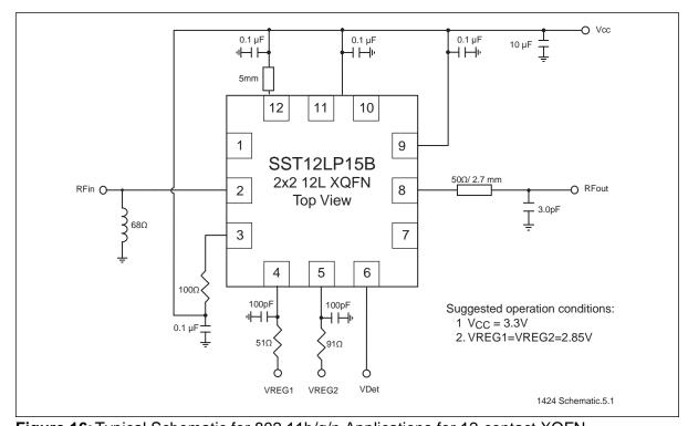
Figure 16: Typical Schematic for 802.11b/g/n Applications for 12-contact XQFN
