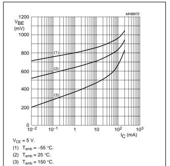
Fig.4 Base-emitter voltage as a function of collector current; typical values.
