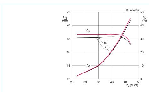
$V_{DS} = 28 \text{ V}; I_{Dq} = 1300 \text{ mA}.$
