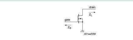
Fig 20. Definition of transistor impedance
