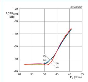
$V_{DS} = 28 \text{ V}; I_{Dq} = 1300 \text{ mA}.$
