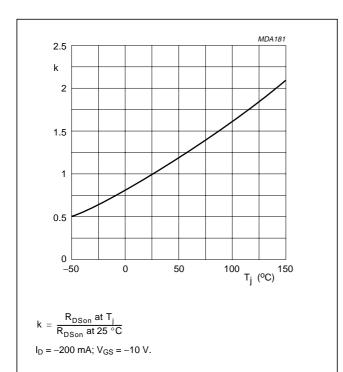
Fig.10 Temperature coefficient of drain-source on-state resistance; typical values.
