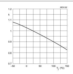
$k \, = \, \frac{V_{GSth} \, \, at \, \, T_j}{V_{GSth} \, \, at \, \, 25^{\circ}C}$
