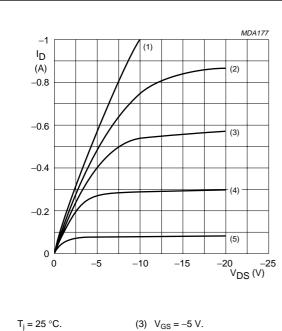
(1)  $V_{GS} = -10 \text{ V}.$
