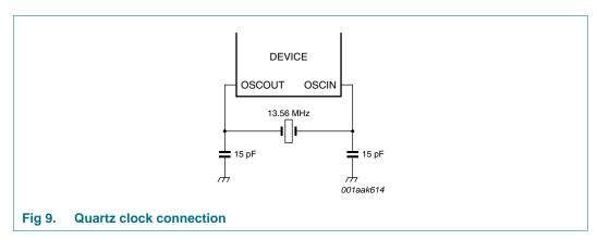
The clock applied to the MFRC500 acts as a time basis for the synchronous system encoder and decoder. The stability of the clock frequency is an important factor for correct operation. To obtain highest performance, clock jitter must be as small as possible. This is best achieved by using the internal oscillator buffer with the recommended circuitry.
