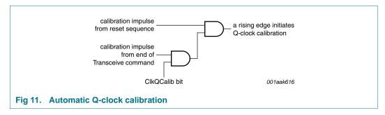
**Remark:** The duration of the automatic Q-clock calibration is 65 oscillator periods or approximately 4.8  $\mu$ s.
