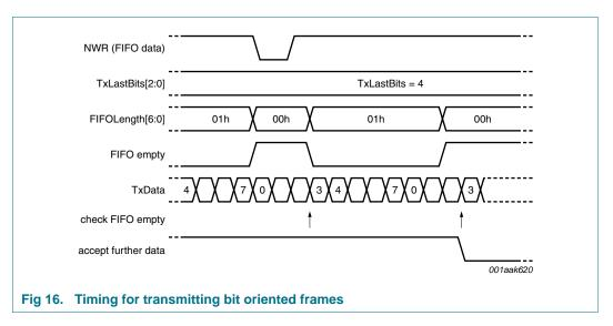
Since in this example TxLastBits[2:0] = 4, transmission stops after bit 3 is transmitted and the frame is completed with an EOF, if configured.
