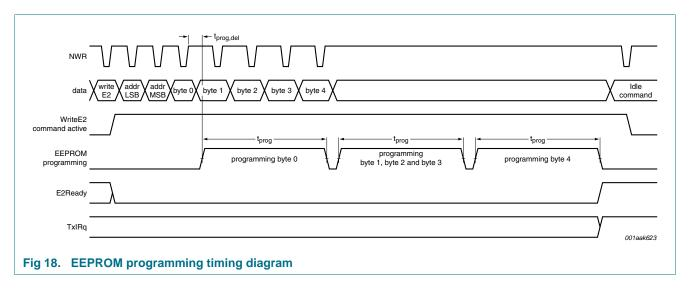
Assuming that the MFRC500 finds and reads byte 0 before the microprocessor is able to write byte 1 ( $t_{prog,del}$  = 300 ns). This causes the MFRC500 to start the programming cycle ( $t_{prog}$ ), which takes approximately 5.8 ms to complete. In the meantime, the microprocessor stores byte 1 to byte 4 in the FIFO buffer.
