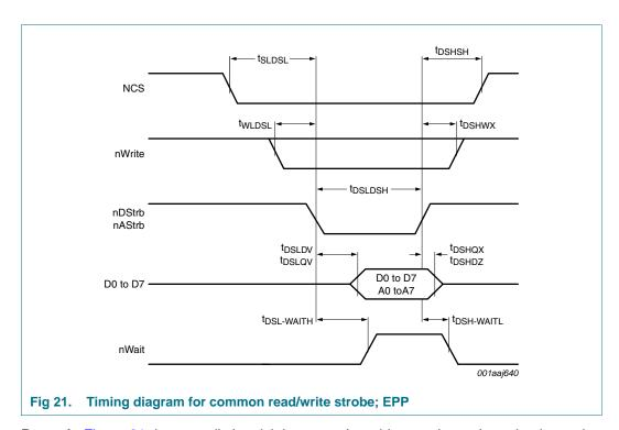
**Remark:** Figure 21 does not distinguish between the address write cycle and a data write cycle. The timings for the address write and data write cycle are different. In EPP mode, the address lines (A0 to A2) must be connected as described in Section 9.1.3 on page 8.
