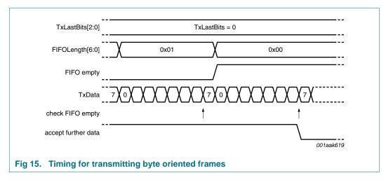
As long as the internal signal accept further data is logic 1, data can be written to the FIFO buffer. The MFRC500 appends this data to the data stream transmitted using the RF interface.
