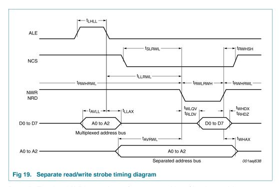
**Remark:** The signal ALE is not relevant for separate address/data bus and the multiplexed addresses on the data bus do not care. The multiplexed address and data bus address lines (A0 to A2) must be connected as described in <u>Section 9.1.3 on page 8</u>.
