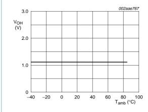
Fig 18.  $V_{OH}$  at  $V_{DD}$  = 3.3 V,  $V_{DD(IO)n}$  = 1.2 V,  $I_{OH}$  = -1 mA
