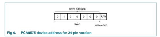
The last bit of the first byte defines the operation to be performed. When set to logic 1 a read is selected, while logic 0 selects a write operation.
