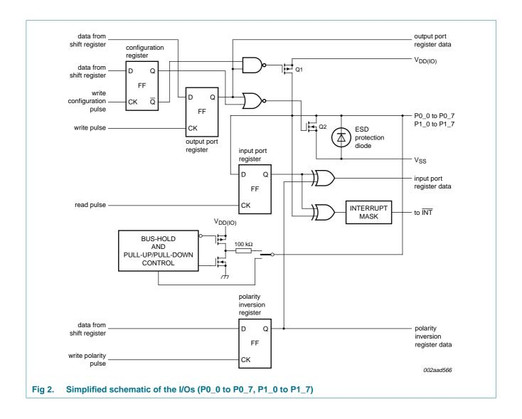
16-bit I<sup>2</sup>C-bus and SMBus, level translating, low voltage GPIO
