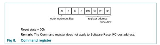
The lowest 4 bits are used as a pointer to determine which register will be accessed. Only a Command register code with the 4 least significant bits equal to the 16 allowable values as defined in <u>Table 3 "Register summary"</u> will be acknowledged. Reserved or undefined command codes will not be acknowledged. At power-up, this register defaults to 00h, with the AI bit set to logic 0, and the lowest 4 bits set to logic 0.
