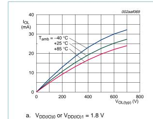
Fig 20. I<sub>OL</sub> versus V<sub>OL</sub>
