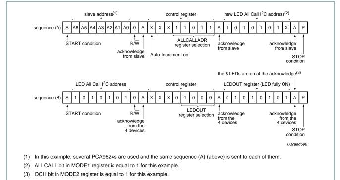
Fig 16. LED All Call I<sup>2</sup>C-bus address programming and LED All Call sequence example
