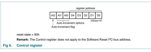
When the Auto-Increment flag is set (AI2 = logic 1), the five low order bits of the Control register are automatically incremented after a read or write. This allows the user to program the registers sequentially. Four different types of Auto-Increment are possible, depending on AI1 and AI0 values.
