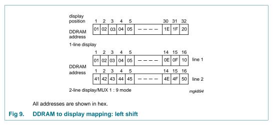
When data is written to or read from the DDRAM, wrap-around occurs from the end of one line to the start of the next line. When the display is shifted each line wraps around within itself, independently of the others. Thus all lines are shifted and wrapped around together. The address ranges and wrap-around operations for the various modes are shown in Table 7.
