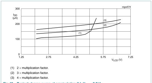
Fig 42. Typical charge pump characteristics (b),  $V_{DD} = 2.7 \text{ V}$
