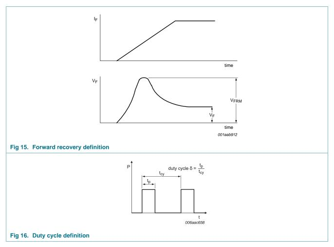
The current ratings for the typical waveforms are calculated according to the equations:  $I_{F(AV)} = I_M \times \delta$  with  $I_M$  defined as peak current,  $I_{RMS} = I_{F(AV)}$  at DC, and  $I_{RMS} = I_M \times \sqrt{\delta}$  with  $I_{RMS}$  defined as RMS current.
