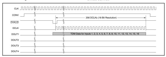
Figure 9. TDM Data Output
