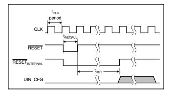
Figure 16. Reset Timing
