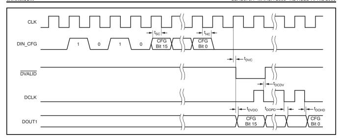
Figure 2. Configuration Register Read/Write Timing
