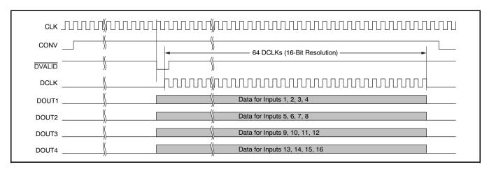
Figure 10. Parallel Data Output
