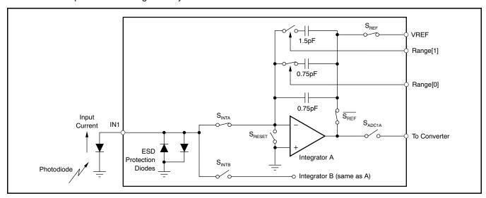
Figure 5. Basic Integration Configuration for Input 1
