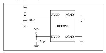
Figure 18. Power-Supply Connections
