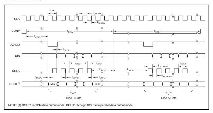
Figure 1. Serial Interface Timing
