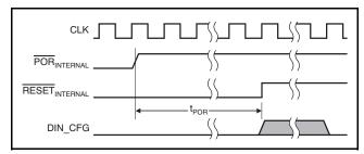
Figure 17. Power-Up Timing
