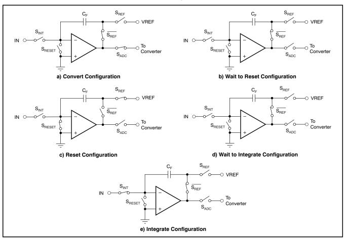
Figure 7. Diagrams for the Five Configurations of DDC316 Front-End Integrators
