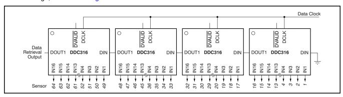
Figure 12. Daisy-Chain Configuration of a 64-Channel System
