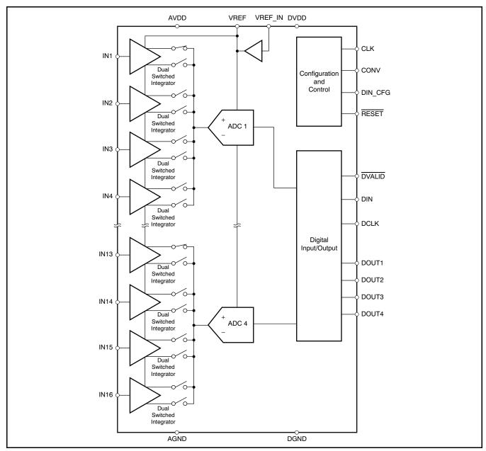
Figure 4. DDC316 Block Diagram
