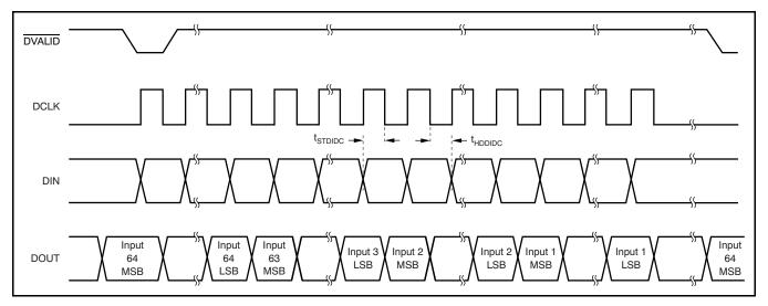
Figure 13. Daisy-Chain Readback of Four Devices (64 Channels)
