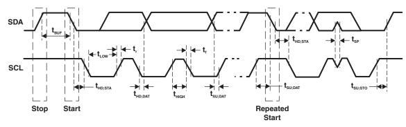
Figure 1. I<sup>2</sup>C Timing
