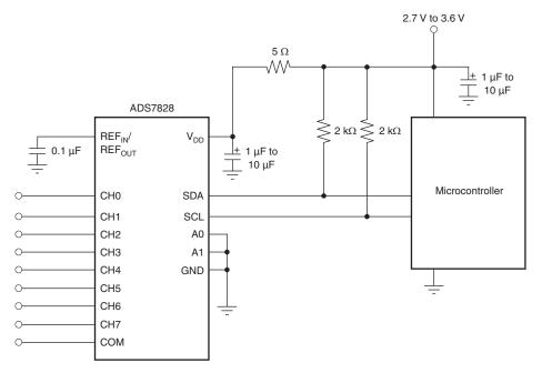
Figure 2. Simplified I/O Diagram
