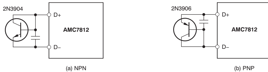
Figure 88. Remote Temperature Sensor Using Transistor
