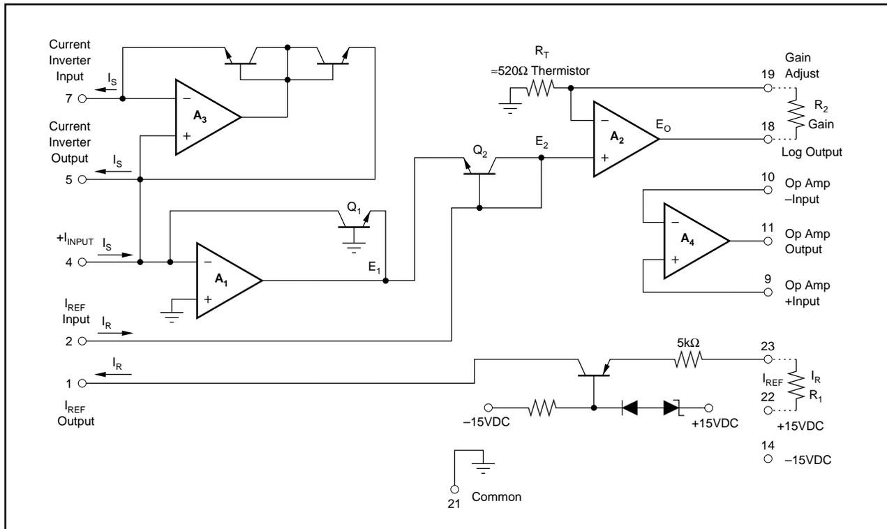
FIGURE 1. Functional Diagram.
