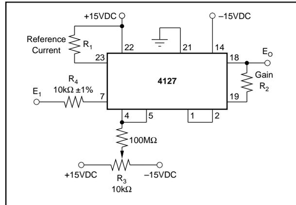
FIGURE 5. Transfer Function When  $E_1$  is Negative.
