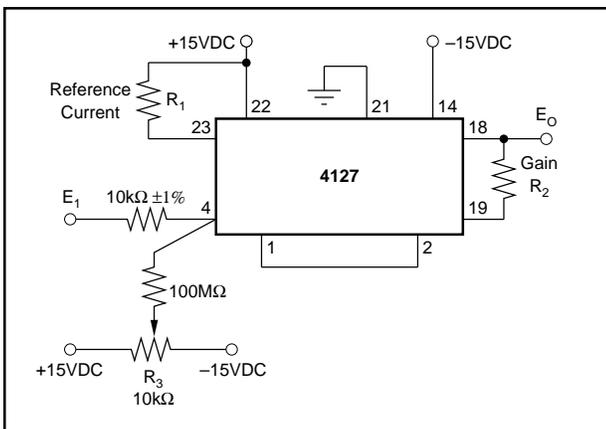
FIGURE 4. Transfer Function When  $E_1$  is Positive.
