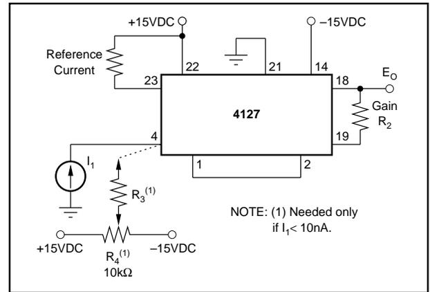
FIGURE 2. Transfer Function When  $I_1$  is Positive.
