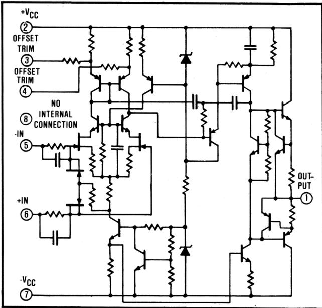
FIGURE 2. Simplified Schematic of 3581 and 3582.
