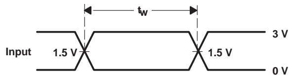
VOLTAGE WAVEFORMS PULSE DURATION
