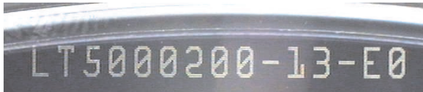
Figure 3-2. Wafer Identification Code 1
