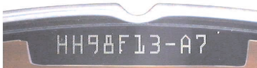
Figure 3-3. Wafer Identification Code 2
