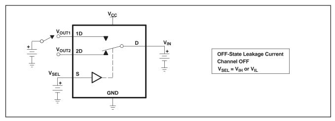
Figure 14. OFF-State Leakage Current
