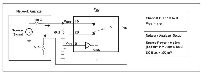
Figure 8. OFF Isolation (O<sub>IRR</sub>)
