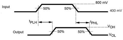
Figure 11. Propagation Delay
