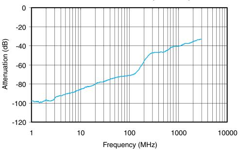
Figure 3. Crosstalk vs Frequency
