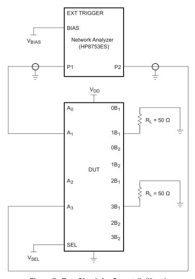
Figure 7. Test Circuit for Crosstalk (X<sub>TALK</sub>)
