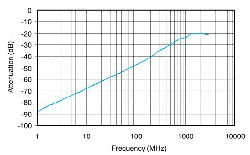
Figure 2. Off Isolation vs Frequency
