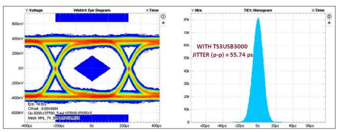
The TS3USB3000 contributes only 3.8ps of peak-to-peak jitter for 2.2 Gbps data rate. Figure 8. Eye Pattern and Time Interval Error Histogram: 2.2 Gbps for MHL Switch
