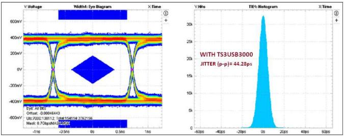
The TS3USB3000 contributes only 8.4ps of peak-to-peak jitter for 0.7 Gbps data rate. Figure 6. Eye Pattern and Time Interval Error Histogram: 0.7 Gbps for MHL Switch
