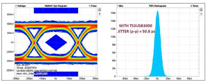
The TS3USB3000 contributes only 5.8ps of peak-to-peak jitter for 3.0 Gbps data rate. Figure 10. Eye Pattern and Time Interval Error Histogram: 3.0 Gbps for MHL Switch
