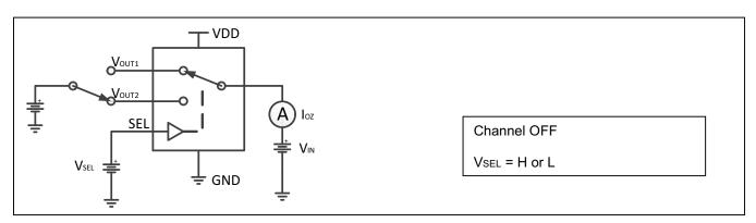
Figure 3. OFF Leakage Current (I<sub>oz</sub>)
