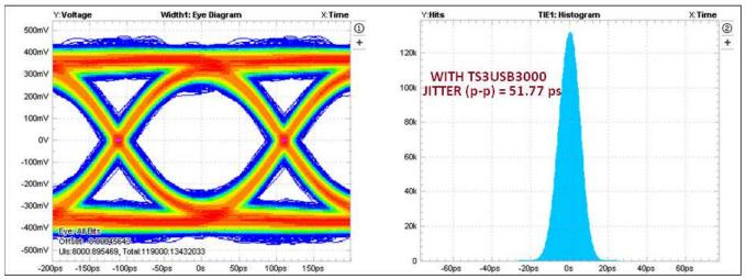
The TS3USB3000 contributes only 7.6ps of peak-to-peak jitter for 4.5 Gbps data rate. Figure 12. Eye Pattern and Time Interval Error Histogram: 4.5 Gbps for MHL Switch
