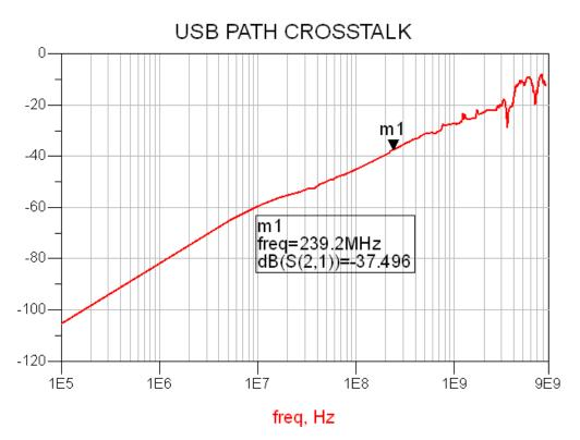
Figure 22. Cross talk vs. Frequency for USB Path
