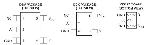
See mechanical drawings for dimensions. DNU - Do not use NC - No internal connection
