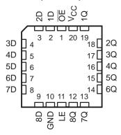
To ensure the high-impedance state during power up or power down,  $\overline{\sf OE}$  should be tied to  ${\sf V}_{\sf CC}$  through a pullup resistor; the minimum value of the resistor is determined by the current-sinking capability of the driver.
