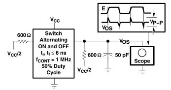
Figure 5. Control to Switch Feedthrough Noise Test Circuit
